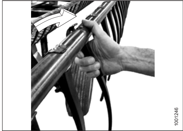
Figure 4.291: Installing Plastic Finger
