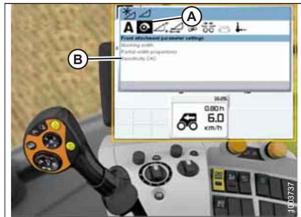
Figure 3.517: CLAAS Lexion Combine Display, Console, and Control Handle
