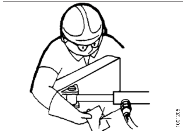
Figure 1.11: Testing for Hydraulic Leaks
