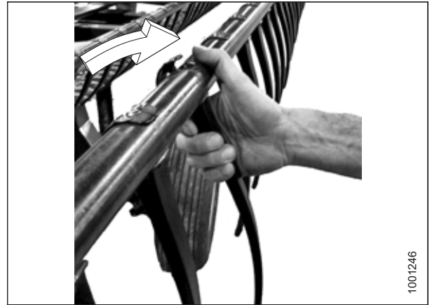
Figure 4.289: Installing Plastic Finger
