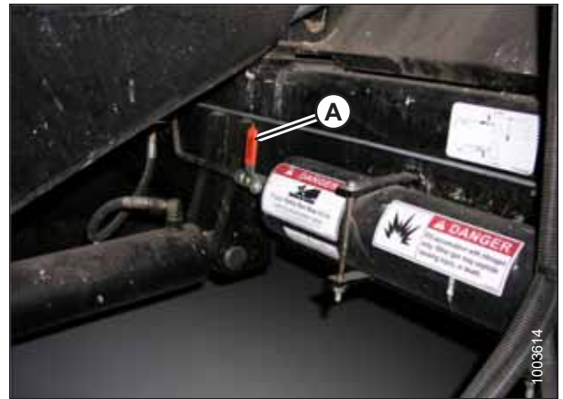
Figure 3.567: Combine Accumulator ON/OFF Switch A - Accumulator Lever (Off Position)
