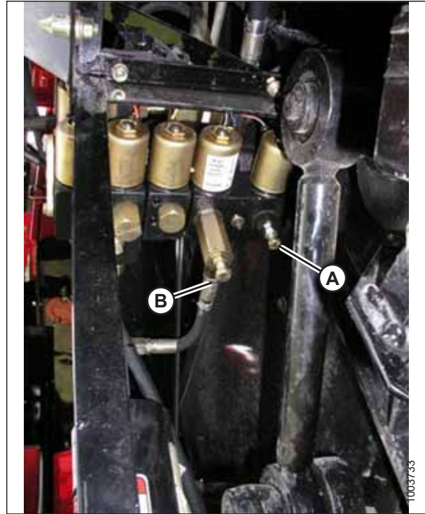
Figure 3.568: Header Raise and Lower Adjustable Restrictors
