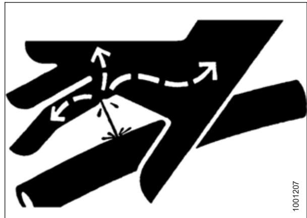
Figure 4.1: Hydraulic Pressure Hazard
