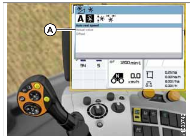
Figure 3.521: CLAAS Lexion Combine Display, Console, and Control Handle
