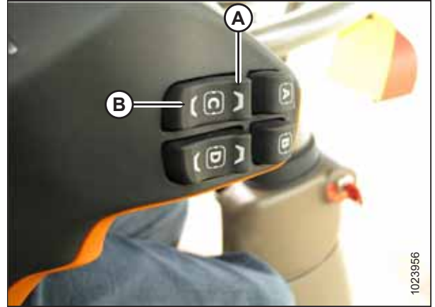
Figure 3.322: John Deere 700 Feeder House Fore-Aft Tilt Controls
