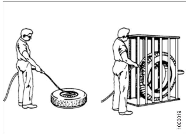
Figure 1.15: Safely Inflating Tire
