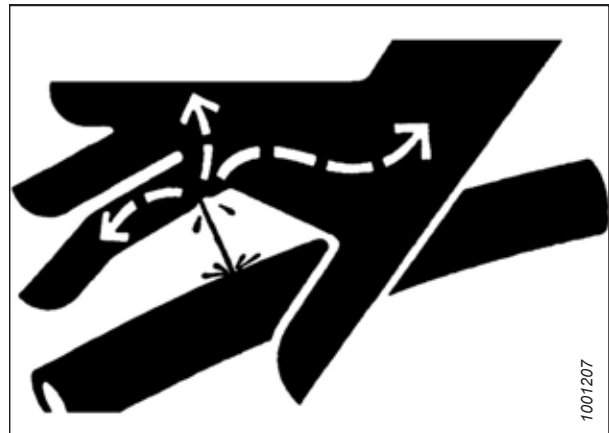
Figure 4.1: Hydraulic Pressure Hazard
