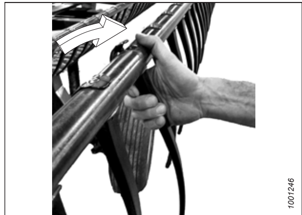
Figure 4.289: Installing Plastic Finger
