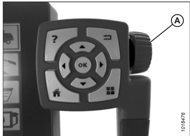
Figure 3.577: Adjustment Wheel on Right Side of Tyton Terminal
