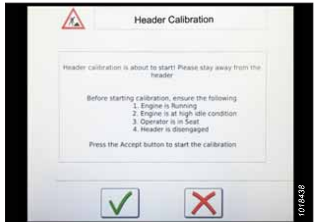
Figure 3.599: Header Calibration Warning
