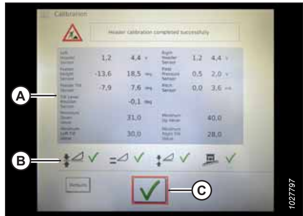
Figure 3.601: Completed Calibration Page
