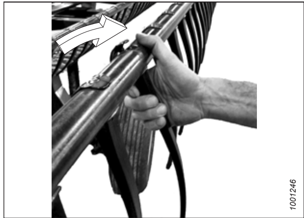
Figure 4.288: Installing Plastic Finger
