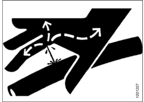
Figure 4.1: Hydraulic Pressure Hazard
