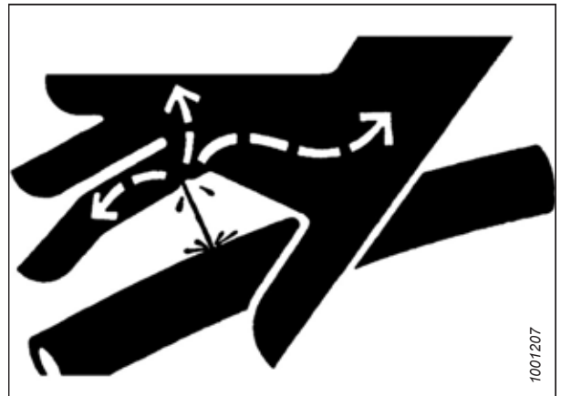
Figure 1.12: Hydraulic Pressure Hazard
