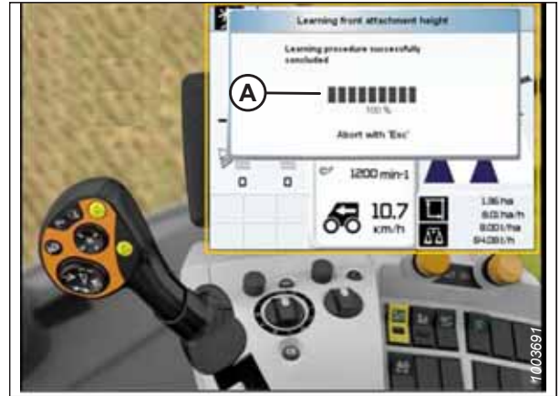
Figure 3.449: CLAAS Combine Display, Console, and Control Handle
