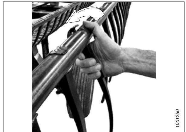
Figure 4.289: Removing Plastic Finger
