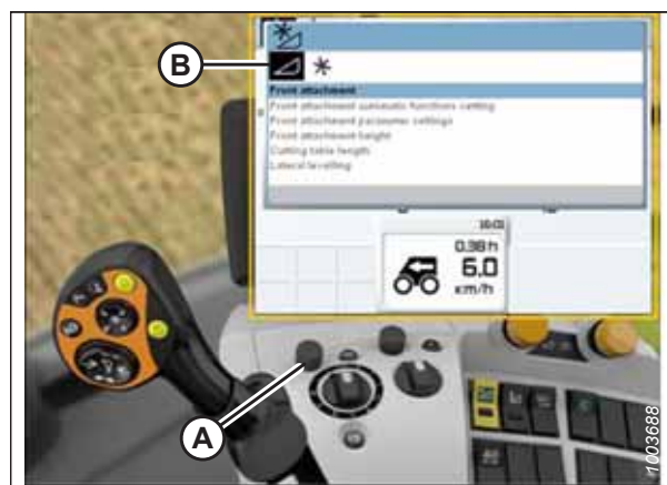
Figure 3.430: CLAAS Combine Display, Console, and Control Handle
