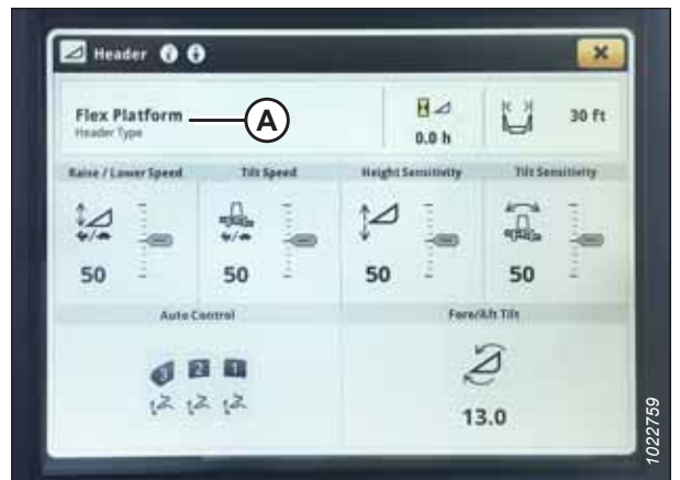
Figure 3.619: John Deere S7 Display – Header Page
