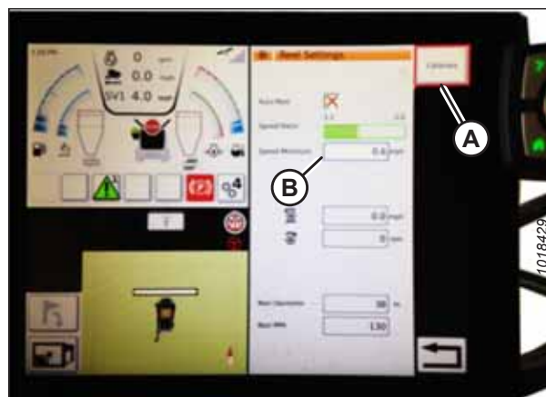
Figure 3.503: Reel Settings Calibration
