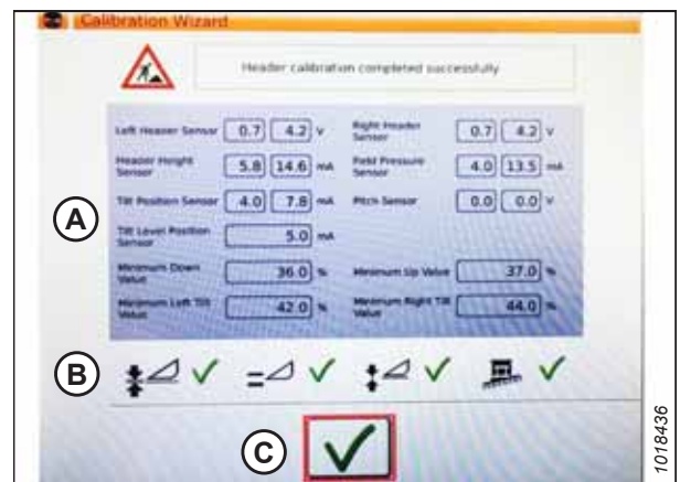
Figure 3.517: Completed Calibration Page
