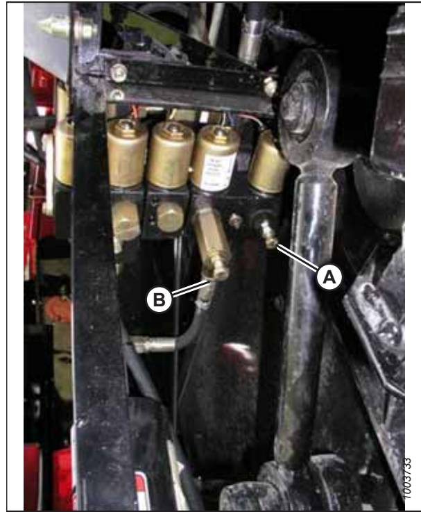
Figure 3.486: Header Raise and Lower Adjustable Restrictors
