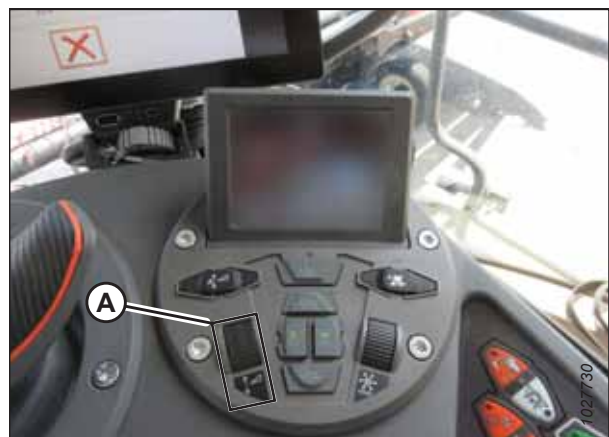
Figure 3.552: Header Control Cluster
