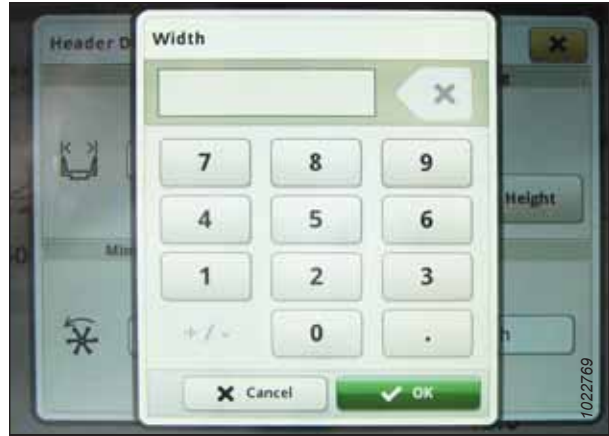
Figure 3.621: John Deere S7 Display – Setting Header Width
