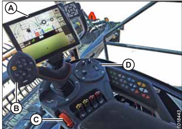
Figure 3.519: Gleaner® S9 Operator Controls
