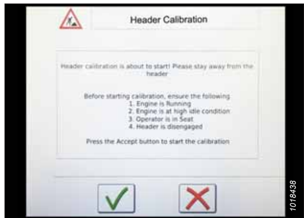
Figure 3.545: Header Calibration Warning
