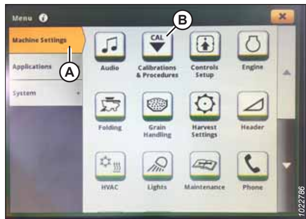
Figure 3.642: John Deere S7 Display – Machine Settings
