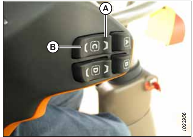
Figure 3.248: John Deere 700 Feeder House Fore-Aft Tilt Controls
