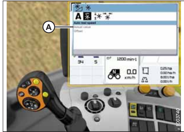
Figure 3.442: CLAAS Combine Display, Console, and Control Handle
