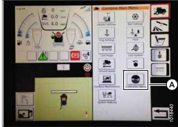
Figure 3.518: Direct Calibration Menu
