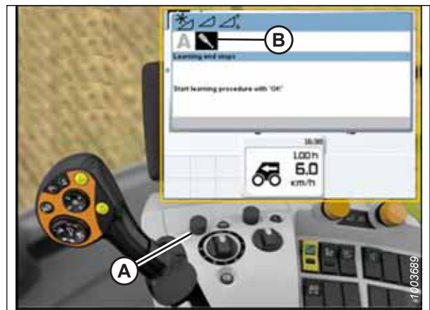
Figure 3.447: CLAAS Combine Display, Console, and Control Handle
