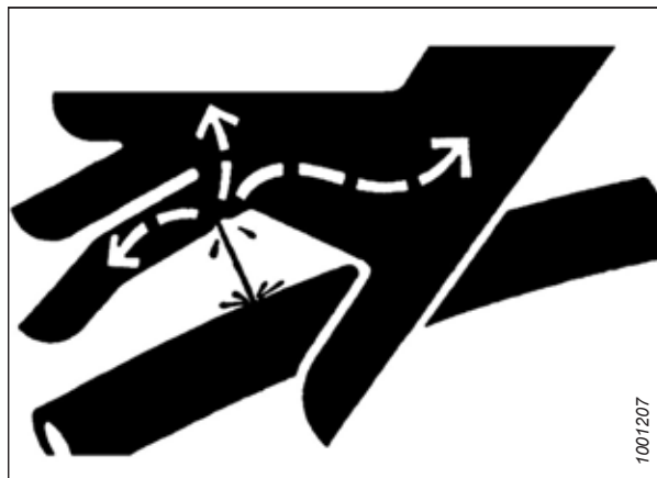
Figure 1.12: Hydraulic Pressure Hazard
