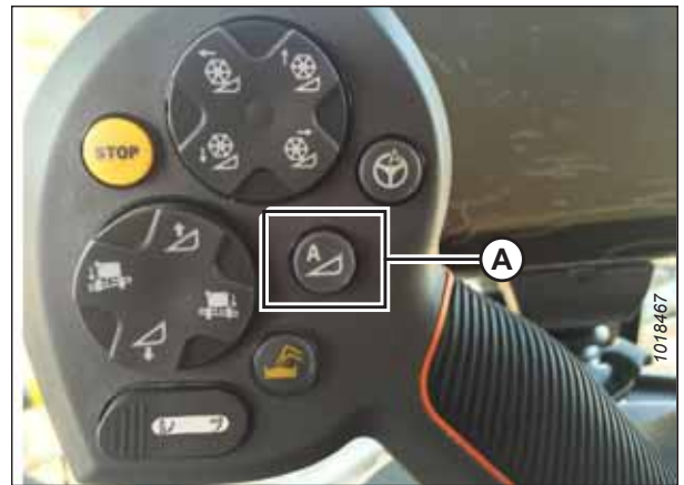
Figure 3.521: AHHC on Control Handle
