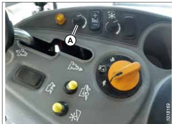
Figure 3.402: Height Adjustment Knob on the Combine Control Console
