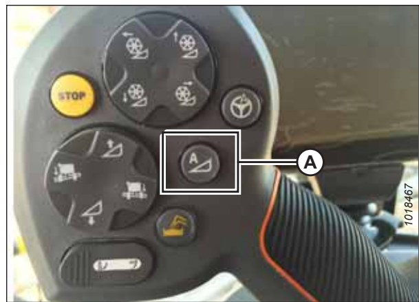
Figure 3.551: AHHC on Control Handle
