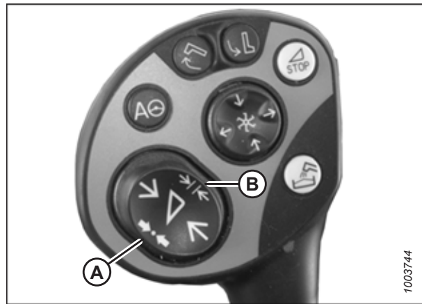
Figure 3.428: CLAAS Control Handle Buttons
