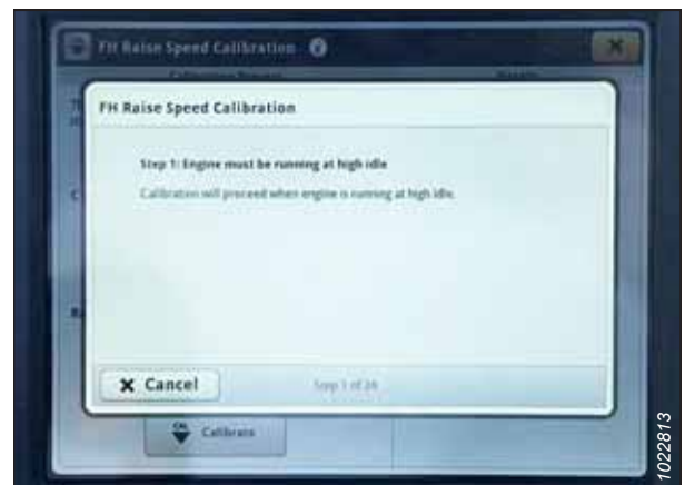
Figure 3.639: John Deere S7 Display – Feeder House Calibration
