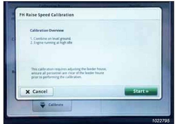
Figure 3.638: John Deere S7 Display – Feeder House Calibration
