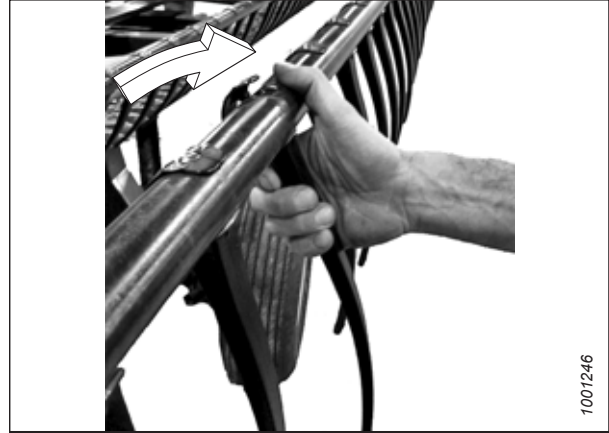
Figure 4.290: Installing Plastic Finger
