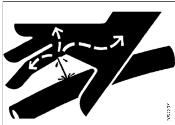
Figure 4.1: Hydraulic Pressure Hazard
