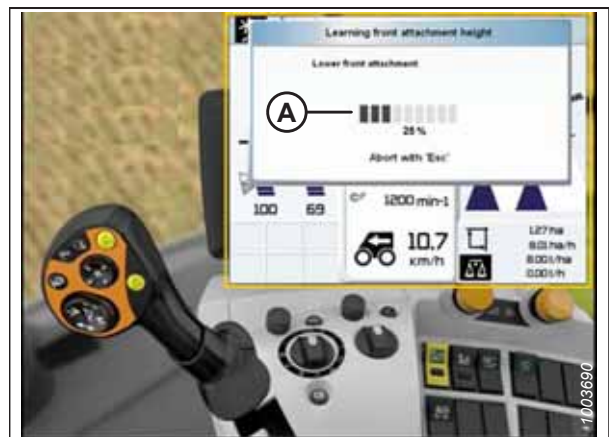
Figure 3.448: CLAAS Combine Display, Console, and Control Handle
