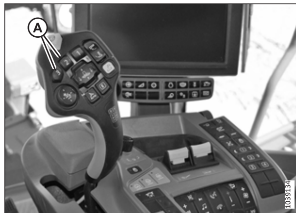
Figure 3.673: John Deere X9 – Multi-Function Lever
