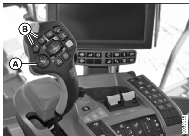
Figure 3.674: John Deere X9 – Multi-Function Lever
