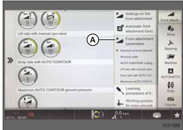
Figure 3.469: Front Attachment Parameters Page
