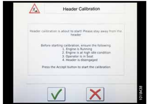
Figure 3.515: Header Calibration Warning
