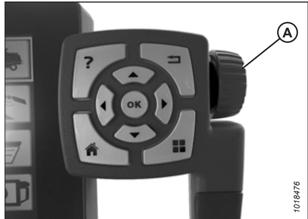
Figure 3.524: Adjustment Wheel on Right Side of Tyton Terminal
