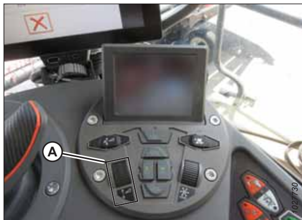
Figure 3.555: Header Control Cluster
