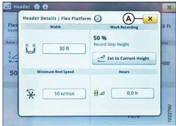
Figure 3.622: John Deere S7 Display – Header Details Dialog Box
