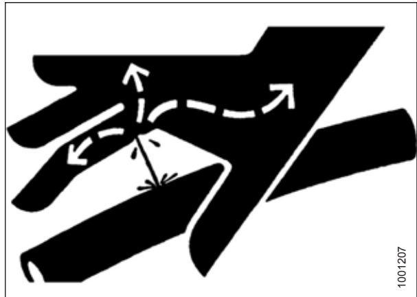
Figure 5.3: Hydraulic Pressure Hazard
