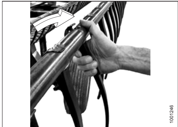
Figure 5.169: Installing Plastic Finger
