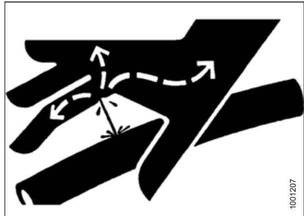
Figure 1.12: Hydraulic Pressure Hazard
