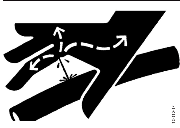
Figure 5.3: Hydraulic Pressure Hazard
