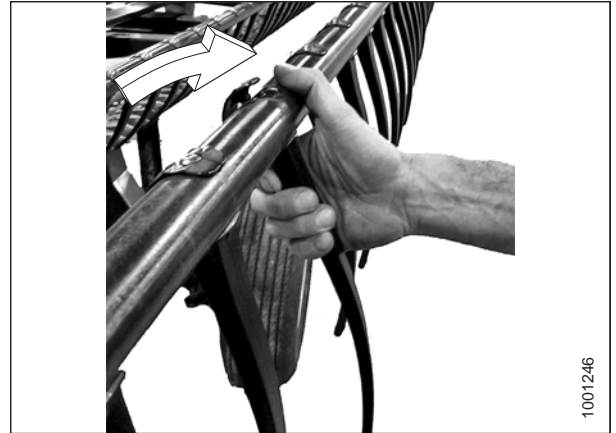
Figure 5.170: Installing Plastic Finger
