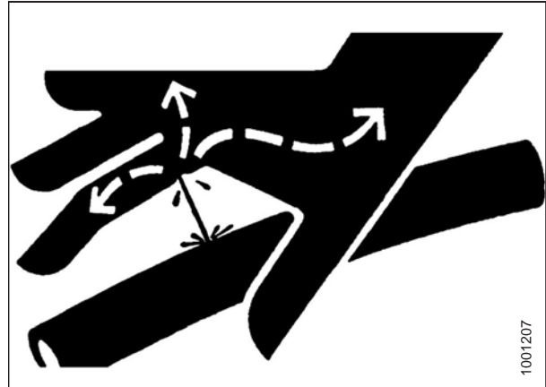
Figure 5.3: Hydraulic Pressure Hazard
