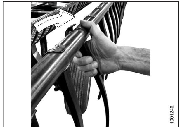
Figure 5.169: Installing Plastic Finger
