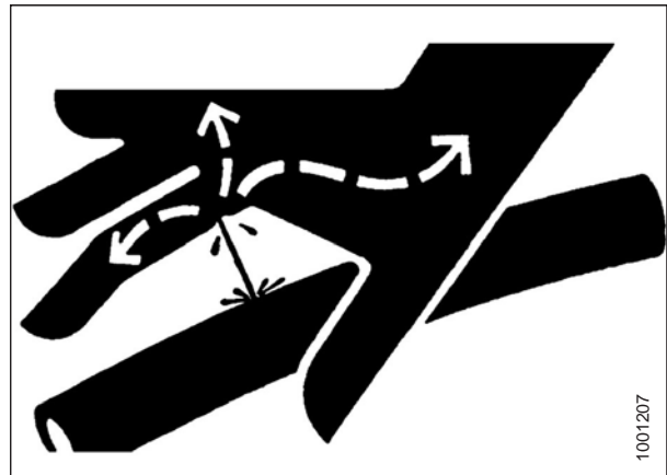
Figure 1.12: Hydraulic Pressure Hazard
