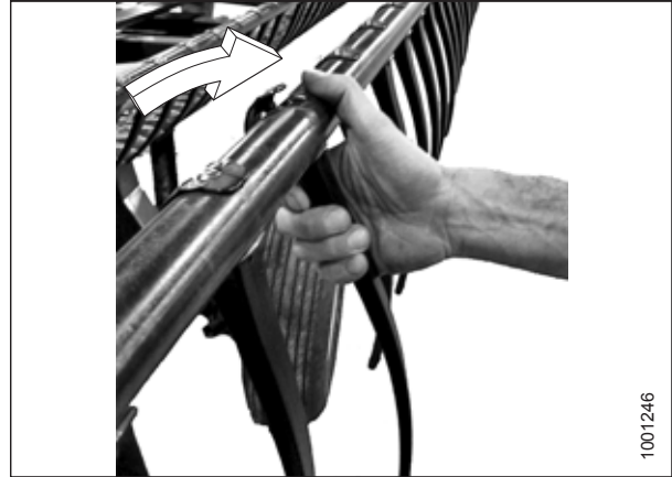
Figure 5.166: Installing Plastic Finger
