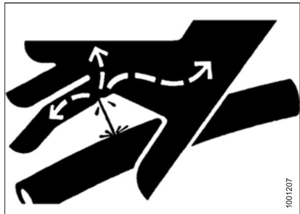
Figure 1.12: Hydraulic Pressure Hazard
