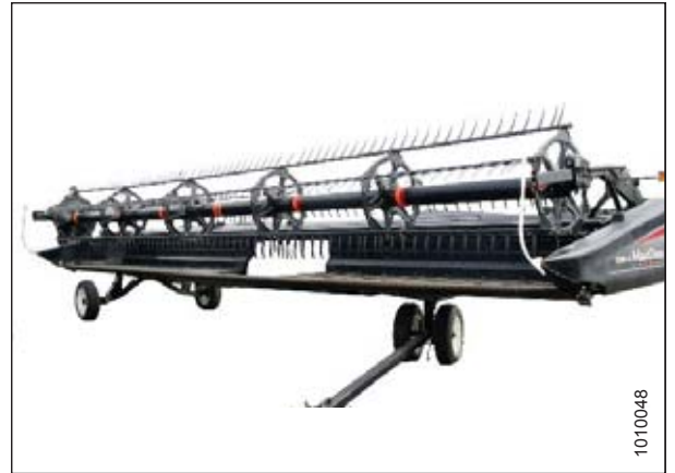
Figure 6.8: Stabilizer Wheels Slow Speed Transport
