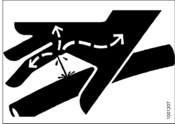
Figure 5.3: Hydraulic Pressure Hazard
