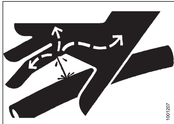
Figure 1.12: Hydraulic Pressure Hazard
