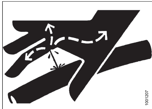
Figure 5.3: Hydraulic Pressure Hazard
