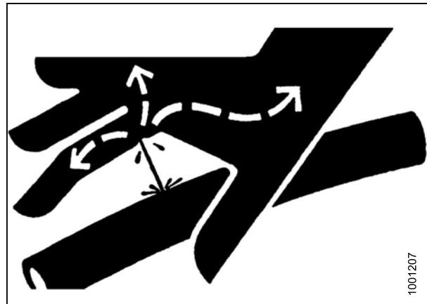
Figure 1.12: Hydraulic Pressure Hazard
