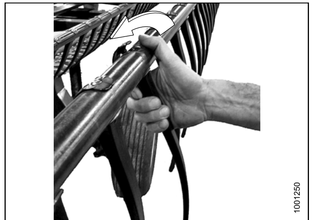
Figure 5.166: Removing Plastic Finger
