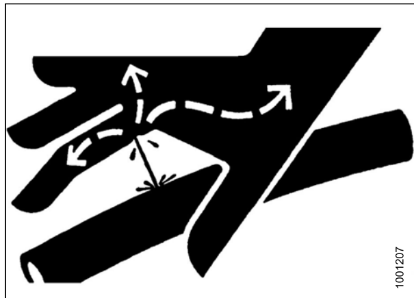
Figure 5.3: Hydraulic Pressure Hazard
