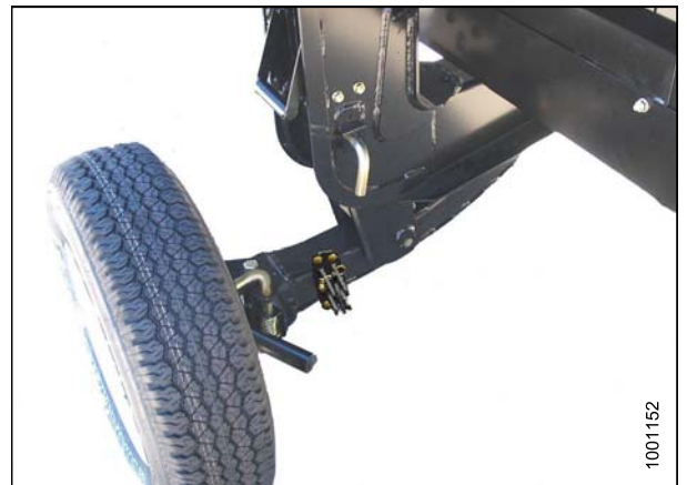
Figure 3.103: Left Wheel in Transport Position
