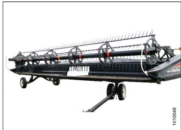
Figure 6.13: Stabilizer Wheels Slow Speed Transport
