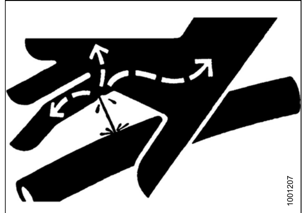
Figure 5.3: Hydraulic Pressure Hazard
