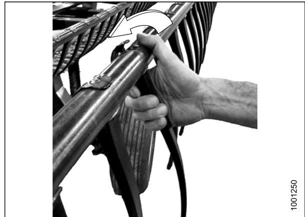
Figure 5.161: Removing Plastic Fingers
