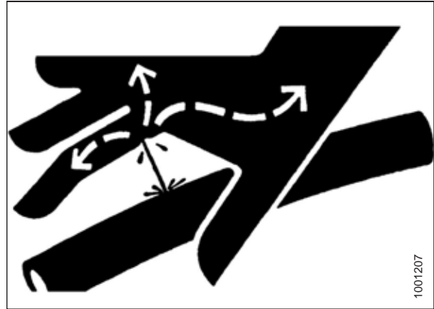
Figure 5.1: Hydraulic Pressure Hazard
