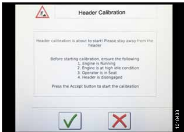
Figure 3.390: Header Calibration Warning
