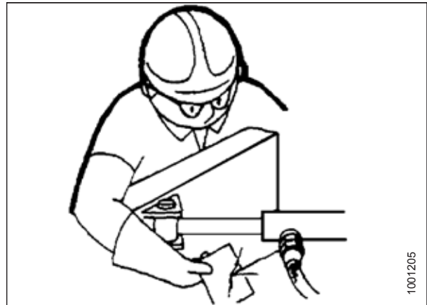
Figure 5.3: Testing for Hydraulic Leaks
