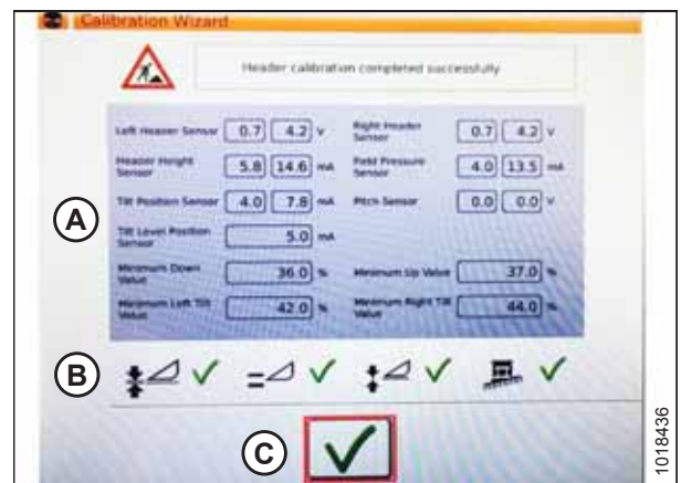
Figure 3.422: Completed Calibration Page
