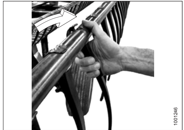
Figure 5.286: Installing Plastic Finger
