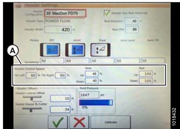
Figure 3.362: Header Speed Control Settings
