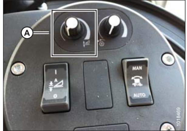
Figure 3.377: Header Control Cluster
