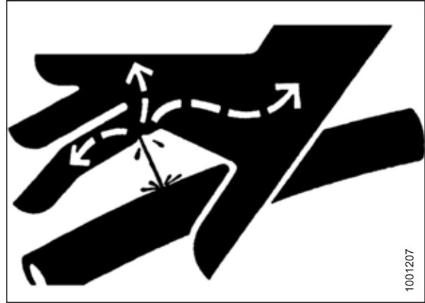
Figure 5.2: Hydraulic Pressure Hazard
