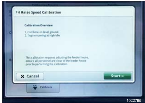
Figure 3.475: John Deere S7 Display – Feeder House Calibration
