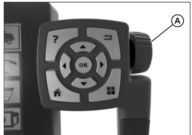
Figure 3.379: Adjustment Wheel on Right Side of Tyton Terminal
