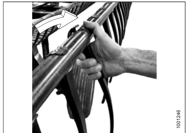
Figure 5.281: Installing Plastic Finger
