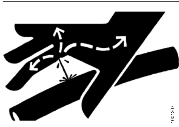
Figure 1.12: Hydraulic Pressure Hazard
