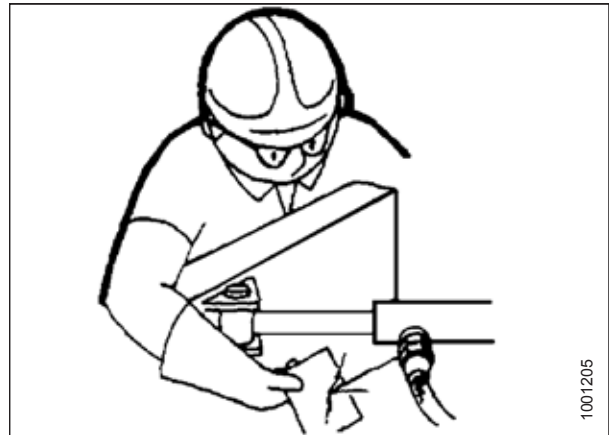
Figure 5.3: Testing for Hydraulic Leaks
