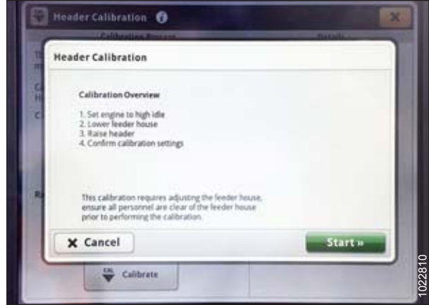
Figure 3.483: John Deere S7 Display – Header Calibration
