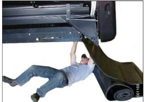
Figure 5.198: Installation du tapis
