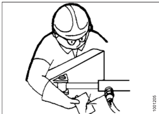
Figure 1.11: Test de fuites hydrauliques
