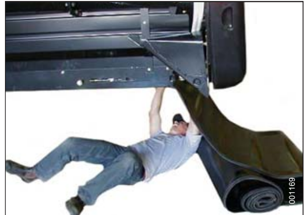
Figure 5.198: Installation du tapis
