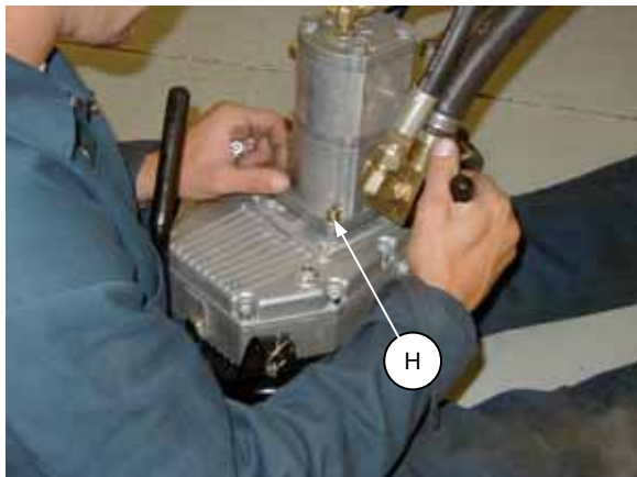
MOUNT PUMP TO GEARBOX
