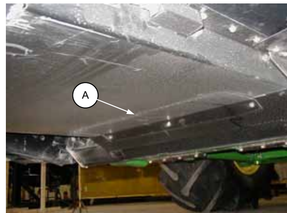
FEED DECK CLEANOUT COVER
