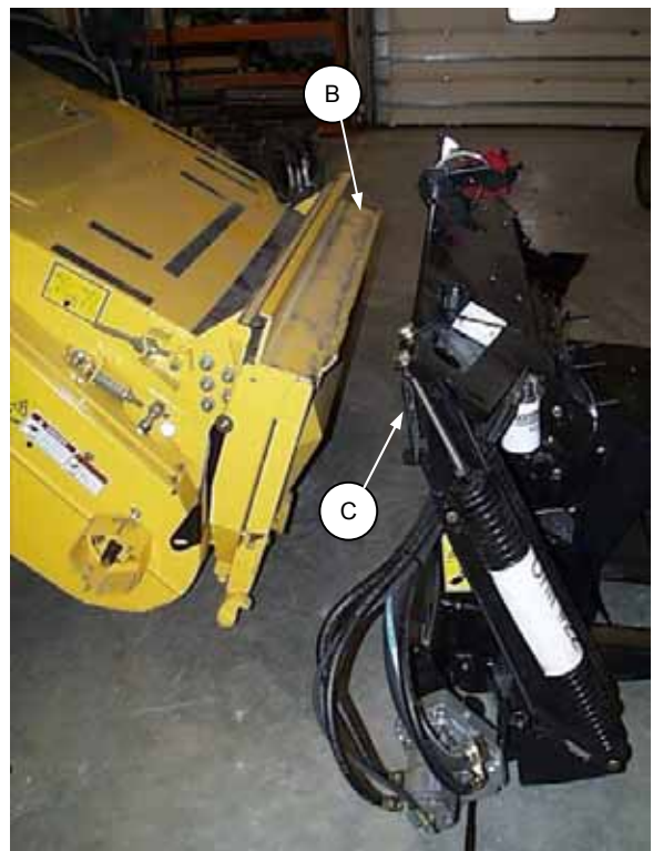
ALIGN FEEDER SADDLE UNDER ADAPTER FRAME – CX SHOWN
