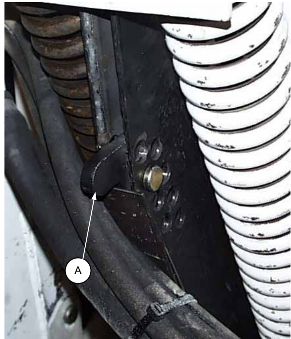
LIMIT FLOAT BY RAISING "ENGAGED" POSITION OF HANDLE
