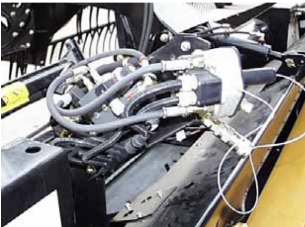
OUTBOARD VIEW COUPLER BRACKET AT L/H LEG (400 SERIES COMBINE COUPLER SHOWN) (500 SERIES COMBINE COUPLERS INCLUDE REEL DRIVE HOSES)
