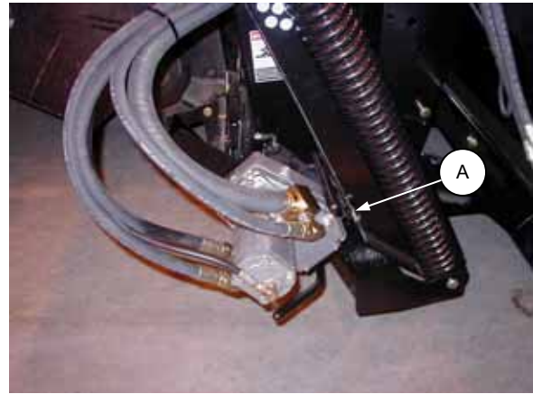
PUMP STORED ON ADAPTER FRAME
