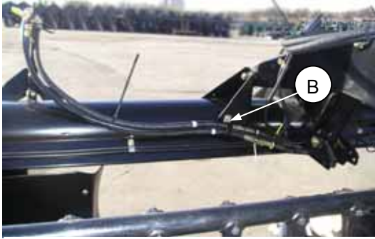
CLAMPING FORE-AFT HOSES - AFTER SETUP
