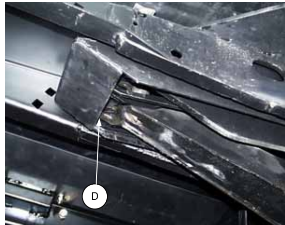
ADAPTER LEG MUST BE ENGAGED IN SUPPORT/CHANNEL – BOTH SIDES
