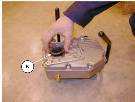
INSTALL WASHER BETWEEN PUMP & GEARBOX
