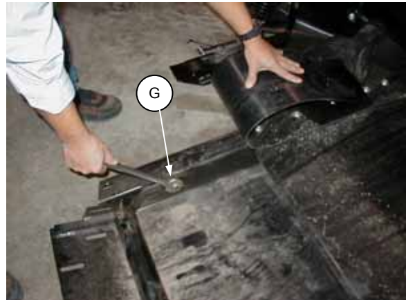
LOOSEN IDLER ROLLER HARDWARE
