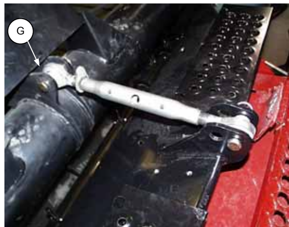
DISCONNECT TOP LINK
