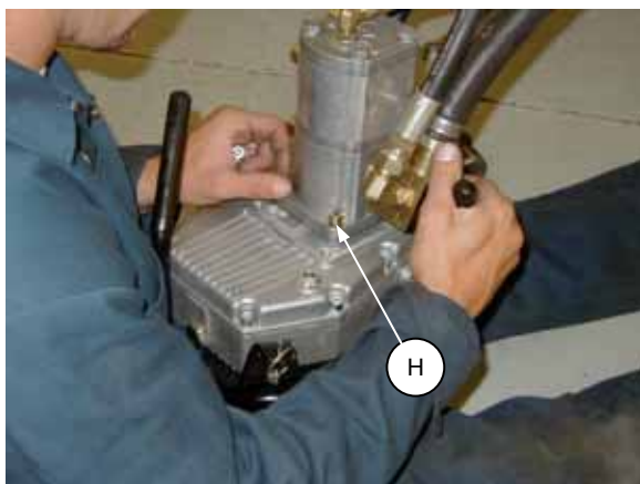
MOUNT PUMP TO GEARBOX
