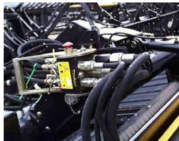
MULTI-LINK CONNECTED TO HEADER
