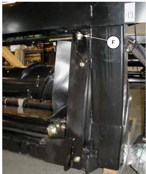
ADJUST ALIGNMENT OF PINS WITH WASHERS
