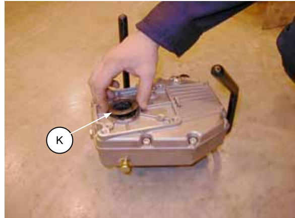
INSTALL WASHER BETWEEN PUMP & GEARBOX
