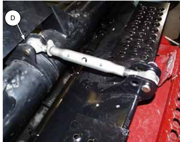
CONNECT TOP LINK BEFORE LIFTING
