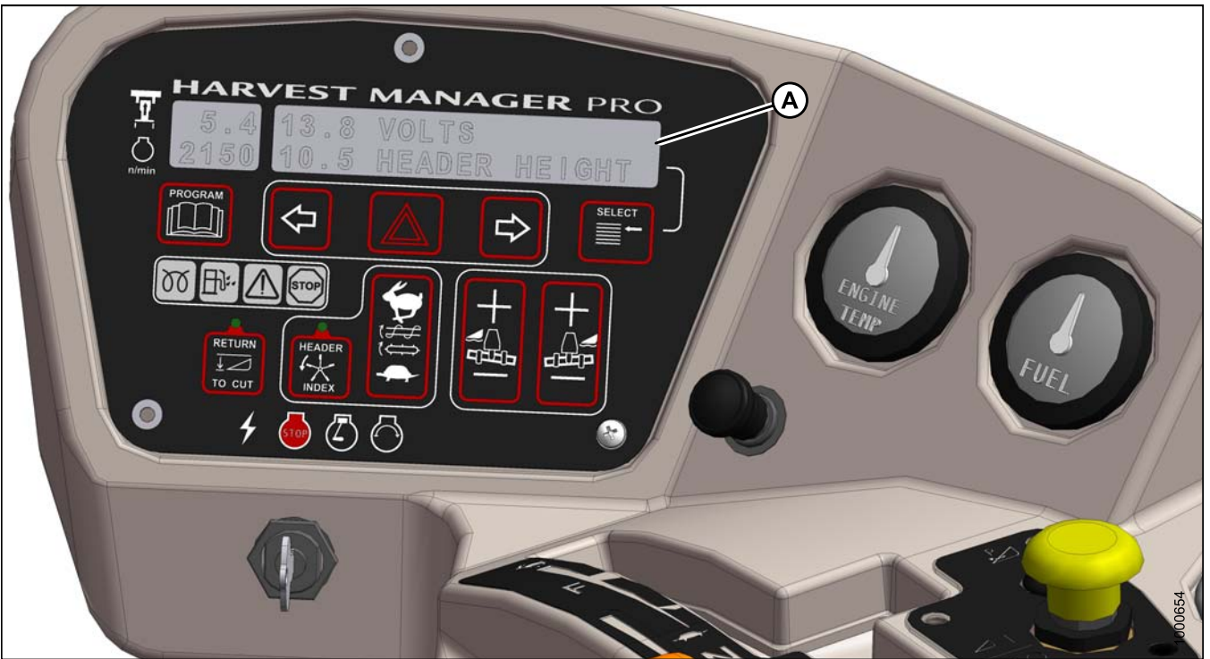
Figure 3.63: CDM Display Warnings and Alarms
