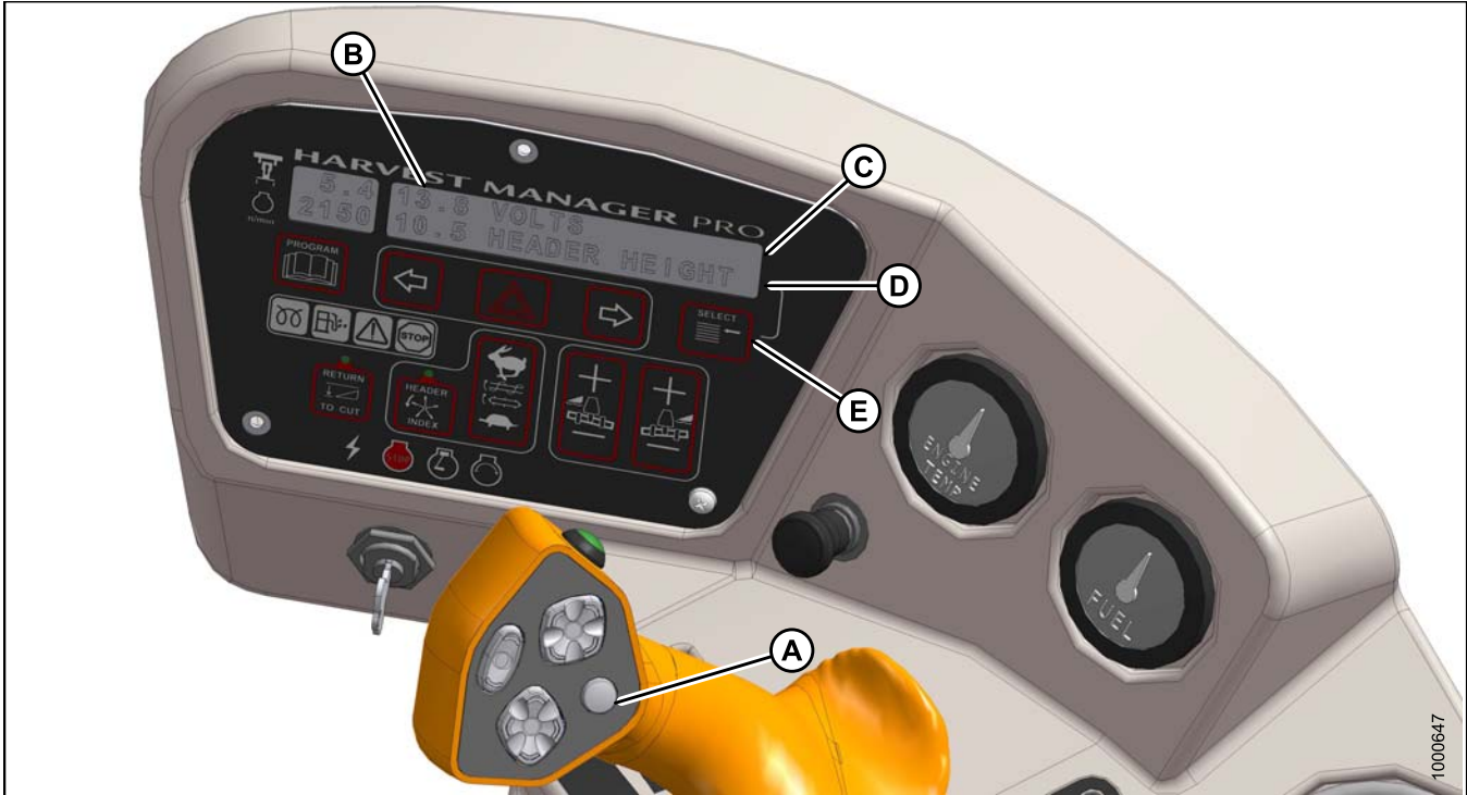
Figure 3.61: CDM Operating Screen
