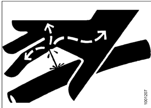
Figure 1.12: Hydraulic Pressure Hazard
