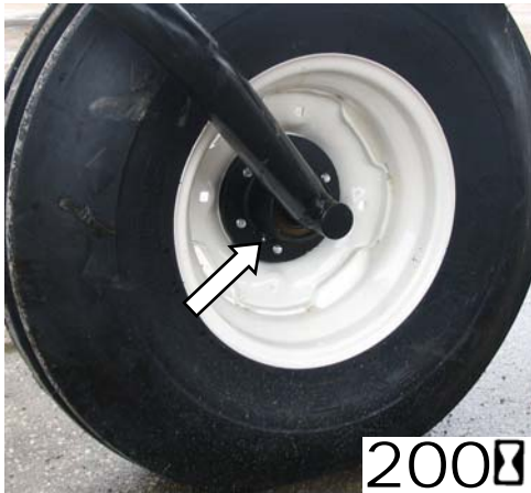
FORMED CASTER WHEEL BEARING 1 PLACE (BOTH WHEELS)
