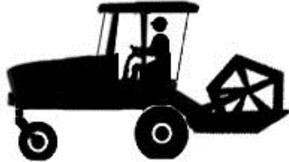
ENGINE FORWARD – SEAT FACES ENGINE ← DIRECTION OF TRAVEL
