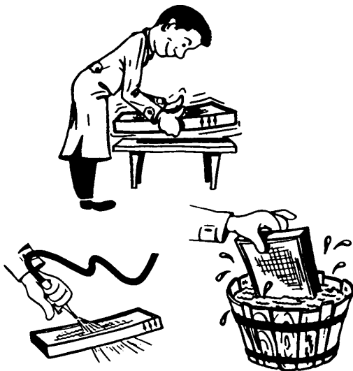
CLEANING AIR FILTER
