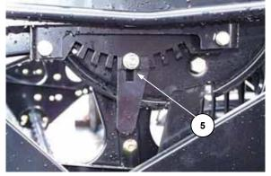
□ Set the fore/aft position to between **4** and **5** on the gauge decal at left reel support arms.
