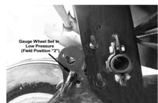
For crop stubble 8" (210mm) or less, set gauge wheels/transport to low pressure (field position "2").
