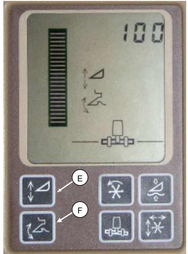
Active header control display
