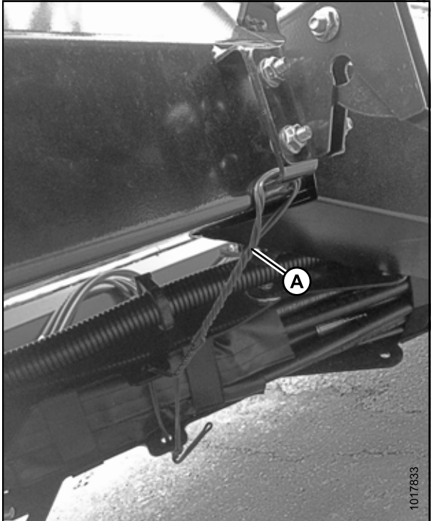
Figure 3.5: Hose Management Arm Shipping Wire
