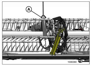
Figure 4.8: Lifting the Reel (Double Reel Only)
