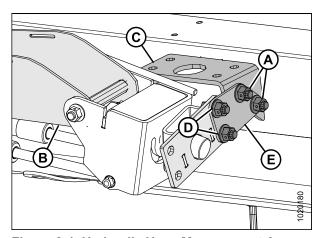
Figure 3.4: Hydraulic Hose Management Arm Base Frame
