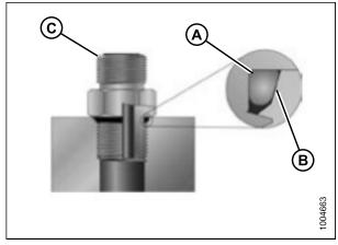
Figure 8.13: Hydraulic Fitting
