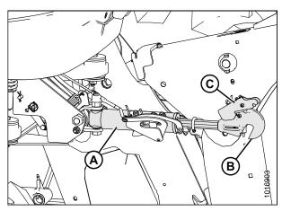
Figure 3.20: Hydraulic Center-Link
