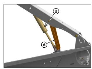
Figure 4.7: Reel Safety Props
