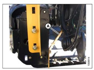
Figure 2.17: Anti-Rotation Brace
