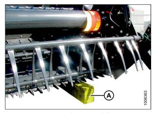
Figure 2.10: Block at One End of Cutterbar
