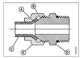
Figure 8.10: Hydraulic Fitting
