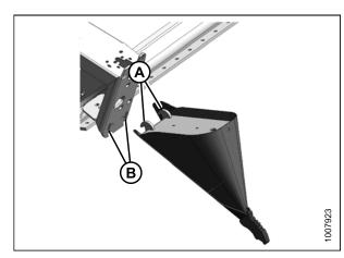
Figure 4.26: Crop Divider Lugs and Endsheet Slots
