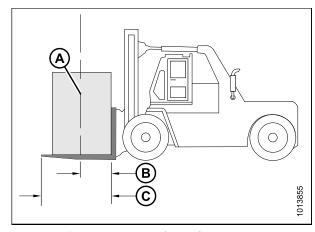
Figure 8.16: Minimum Lifting Capacity
