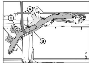
Figure 3.3: Hydraulic Hose Management Arm in Shipping Position
