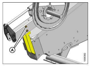
Figure 4.4: Outboard Reel Arm Support
