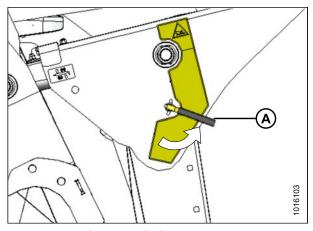
Figure 3.23: Cylinder Safety Prop
