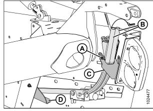
Figure 4.24: Divider Rods on Endsheet
