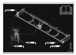
Figure 5.43: Single-Knife Header Grease Point Layout Decal
