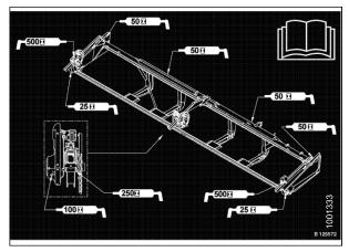
Figure 5.44: Double-Knife Header Grease Point Layout Decal
