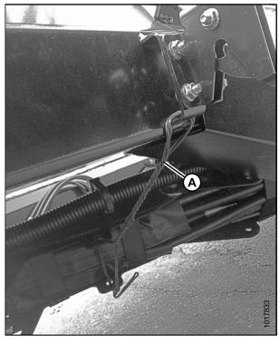
Figure 3.6: Hose Management Arm in Shipping Position (12.2–13.7 Meter [40–45 Foot] Headers)
