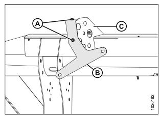
Figure 3.9: Hose Management Arm Shipping Support Bracket (7.6–10.6 Meter [25–35 Foot] Headers)
