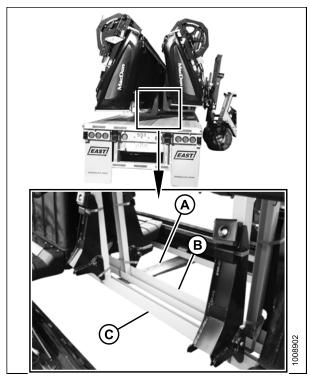
Figure 2.2: Header Shipping Supports
