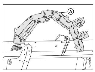
Figure 3.7: Hose Management Arm in Field Position
