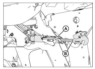
Figure 3.21: Hydraulic Center-Link
