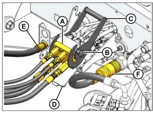
Figure 3.30: Draper/Reel Multicoupler
