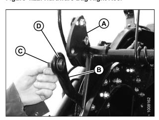
Figure 4.23: Bar Crank Attachment Holes and Link Alignment
