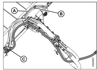
Figure 3.10: Hose Management Arm Hose Routing (Top View)
