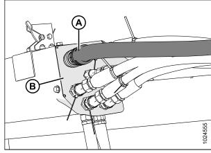
Figure 3.1: Hoses and Connector Attached to the Header
