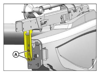
Figure 4.14: Outboard Reel Arm Supports
