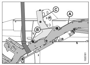
Figure 3.5: Hydraulic Hose Management Arm in Shipping Position (7.6–10.6 Meter [25–35 Foot] Headers)
