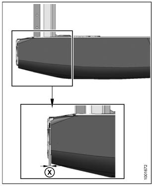
Figure 5.34: Gap between Endshield and Header Frame
