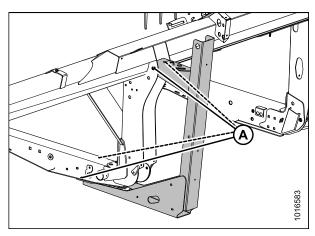
Figure 2.16: Outer Leg Shipping Supports
