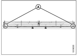
Figure 5.13: Double Reel Measurement Locations
