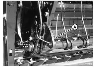
Figure 4.21: Disconnected Cam Links and Shipping Wire
