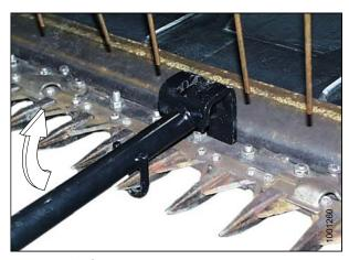
Figure 7.2: Straightening Tool – Upward Adjustment
