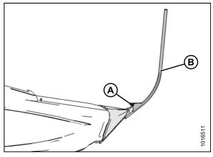
Figure 4.28: Divider Rod on Crop Divider
