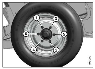
Figure 5.1: Bolt Tightening Sequence
