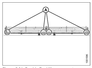
Figure 5.31: Double Reel Measurement **Locations (Four Places)**
