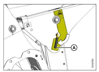
Figure 3.25: Cylinder Safety Prop
