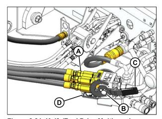
Figure 3.31: Knife/Reel Drive Multicoupler
