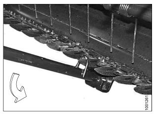
Figure 7.3: Straightening Tool– Downward Adjustment
