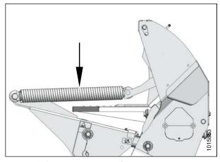
Figure 3.15: Header Float Springs
