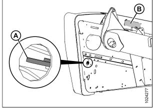
Figure 5.2: Endshield Latch Access
