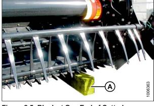
Figure 2.5: Block at One End of Cutterbar
