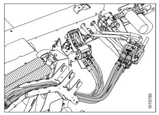
Figure 3.33: Hydraulic Multicouplers and Hose Routing
