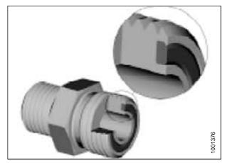
Figure 8.14: Hydraulic Fitting
