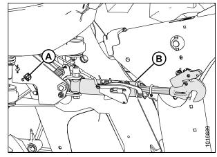
Figure 3.13: Center-Link without Self-Alignment
