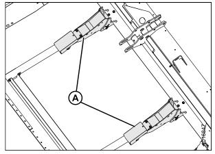
Figure 2.12: Draper Header Supports, and Shipping Supports
