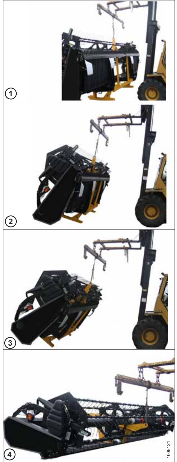
Figure 2.10: Lowering the Header
