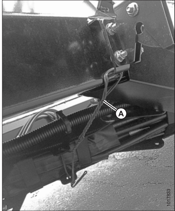
Figure 4.7: Hydraulic Hose Management System in Shipping Position – 12.2–13.7 m (40–45 ft.) Headers
