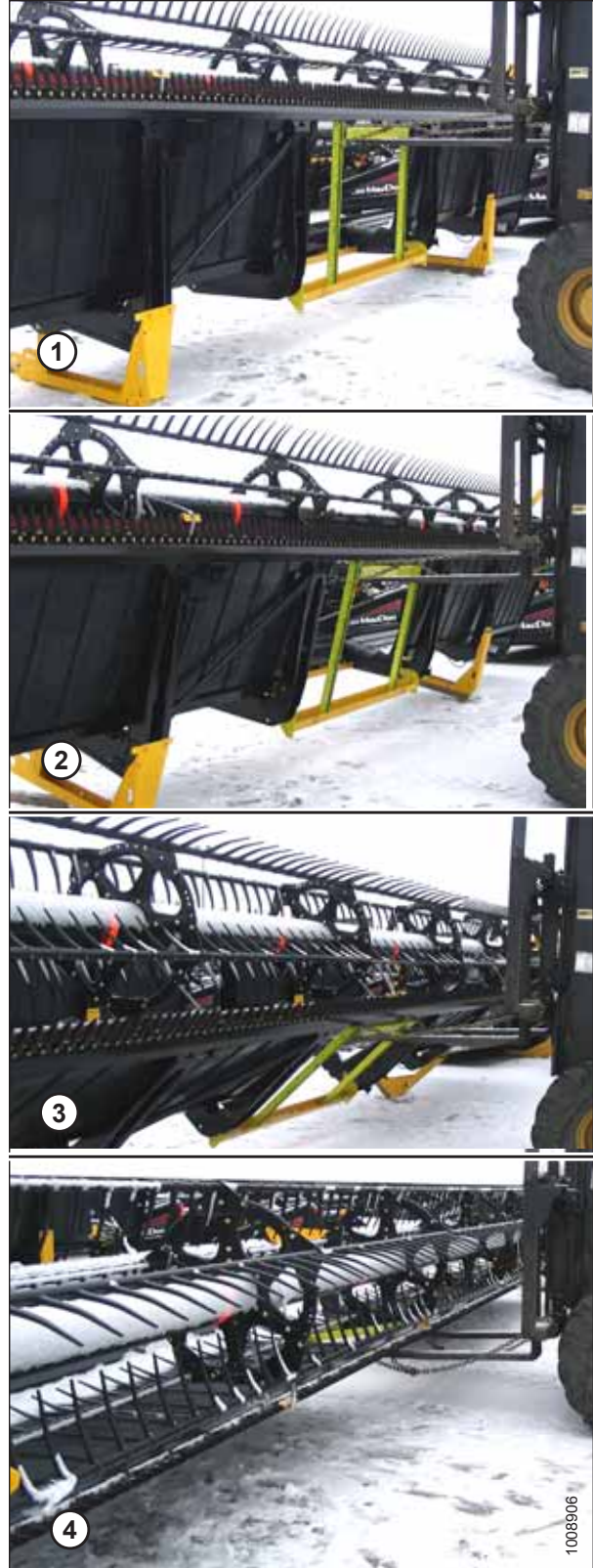
Figure 2.4: Lowering the Header
