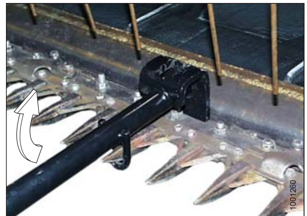
Figure 7.2: Straightening Tool – Upward Adjustment
