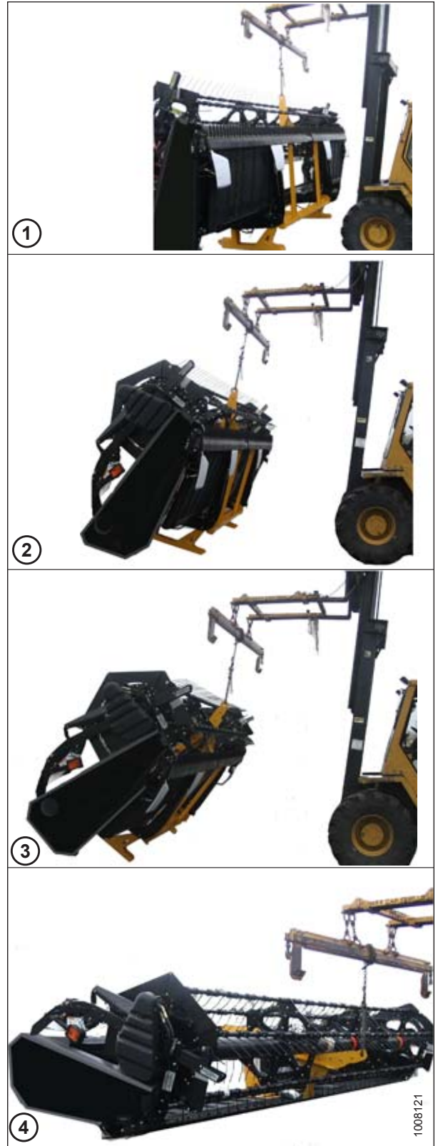
Figure 2.9: Lowering the Header
