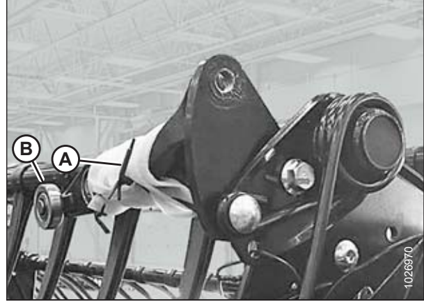
Figure 4.25: Cam Arm in Shipping Position
