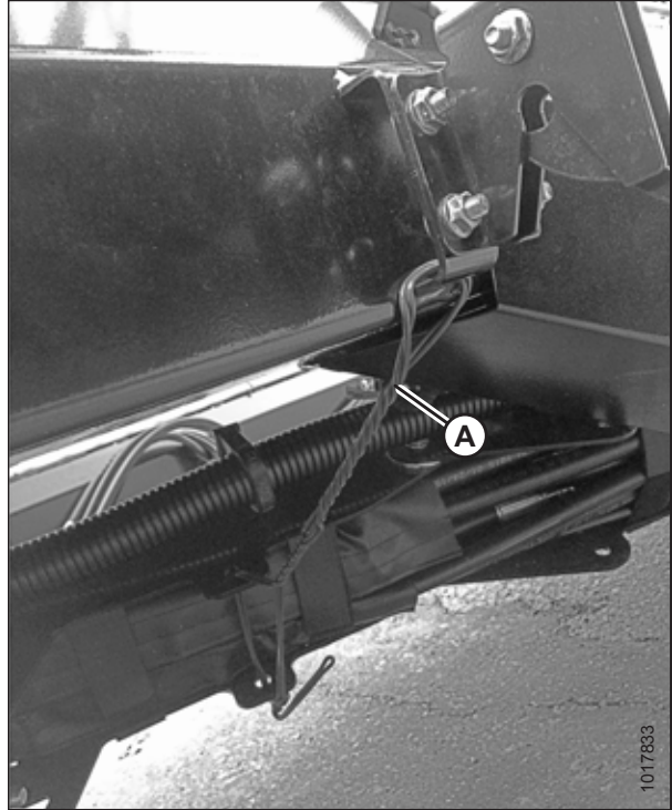
Figure 3.8: Hose Management Arm in Shipping Position – 12.2–13.7 m (40–45 ft.) Headers
