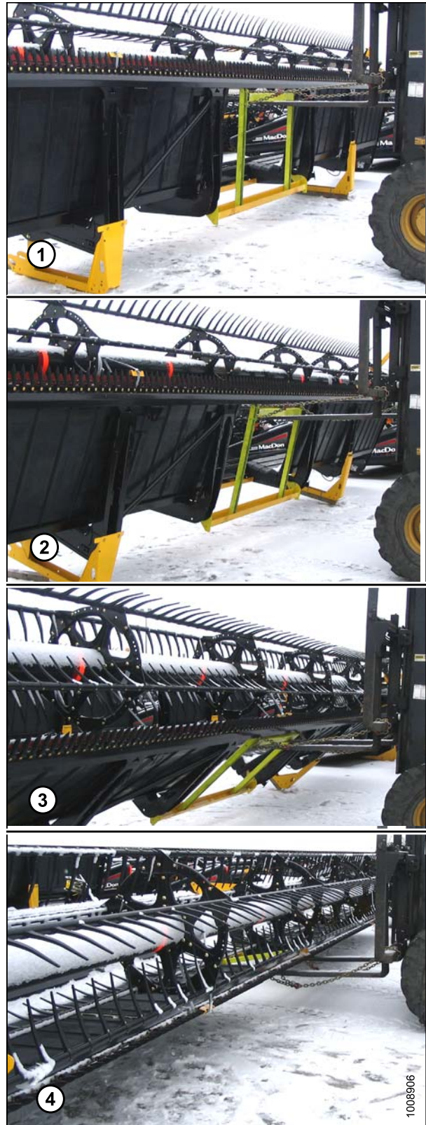
Figure 2.4: Lowering the Header
