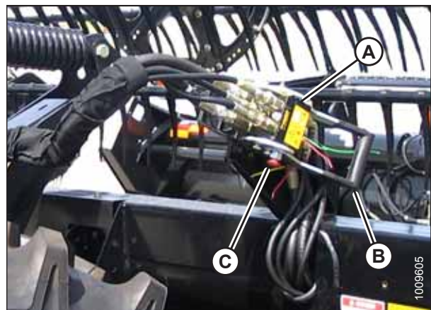
Figure 4.31: Multicoupler on Header
