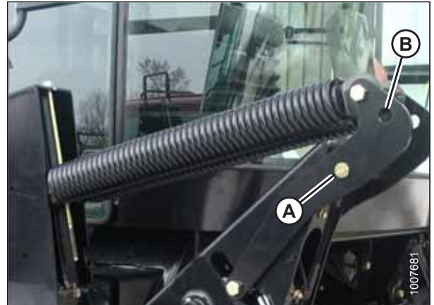
Figure 4.10: Float Springs Engaged
