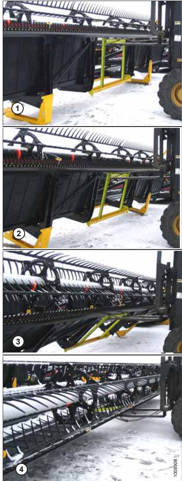
Figure 2.3: Lowering the Header
