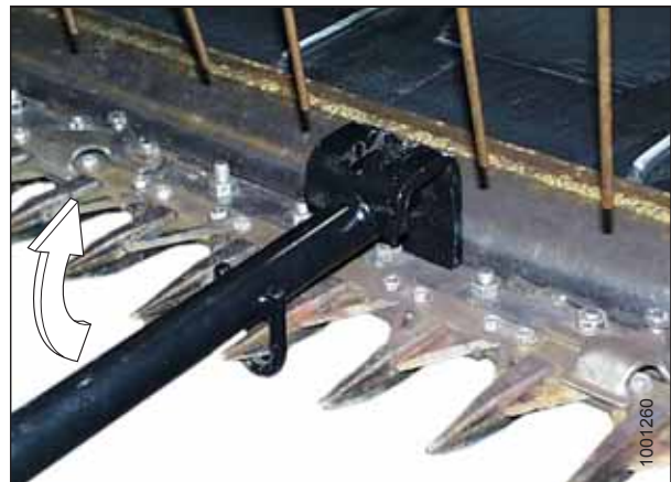
Figure 6.2: Straightening Tool – Upward Adjustment
