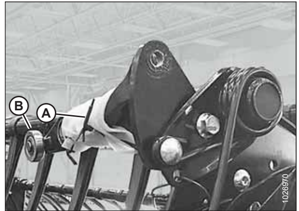
Figure 3.23: Cam Arm in Shipping Position
