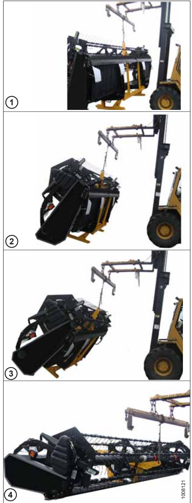
Figure 2.9: Lowering the Header
