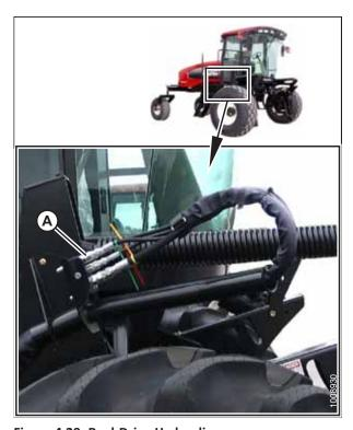
Figure 4.29: Reel-Drive Hydraulics
