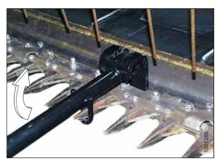
Figure 6.2: Straightening Tool – Upward Adjustment
