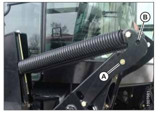
Figure 4.10: Float Springs Engaged
