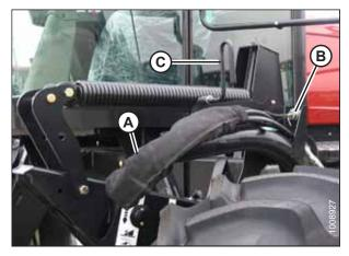
Figure 4.25: Header-Drive Hydraulics and Electrical Harness
