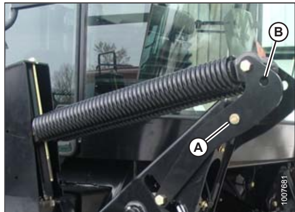
Figure 4.10: Float Springs Engaged
