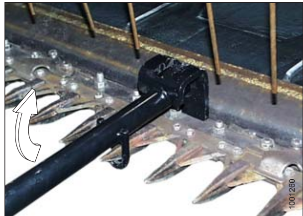
Figure 6.2: Straightening Tool – Upward Adjustment
