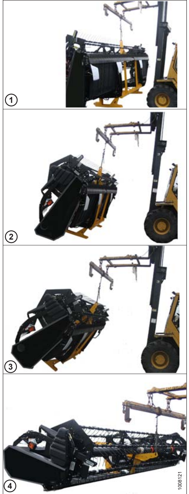
Figure 2.9: Lowering the Header
