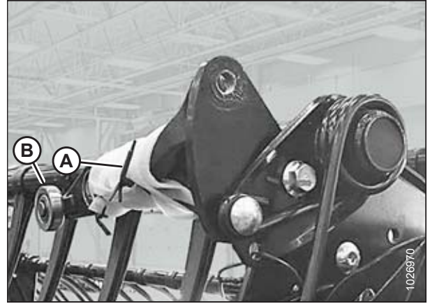
Figure 3.22: Cam Arm in Shipping Position
