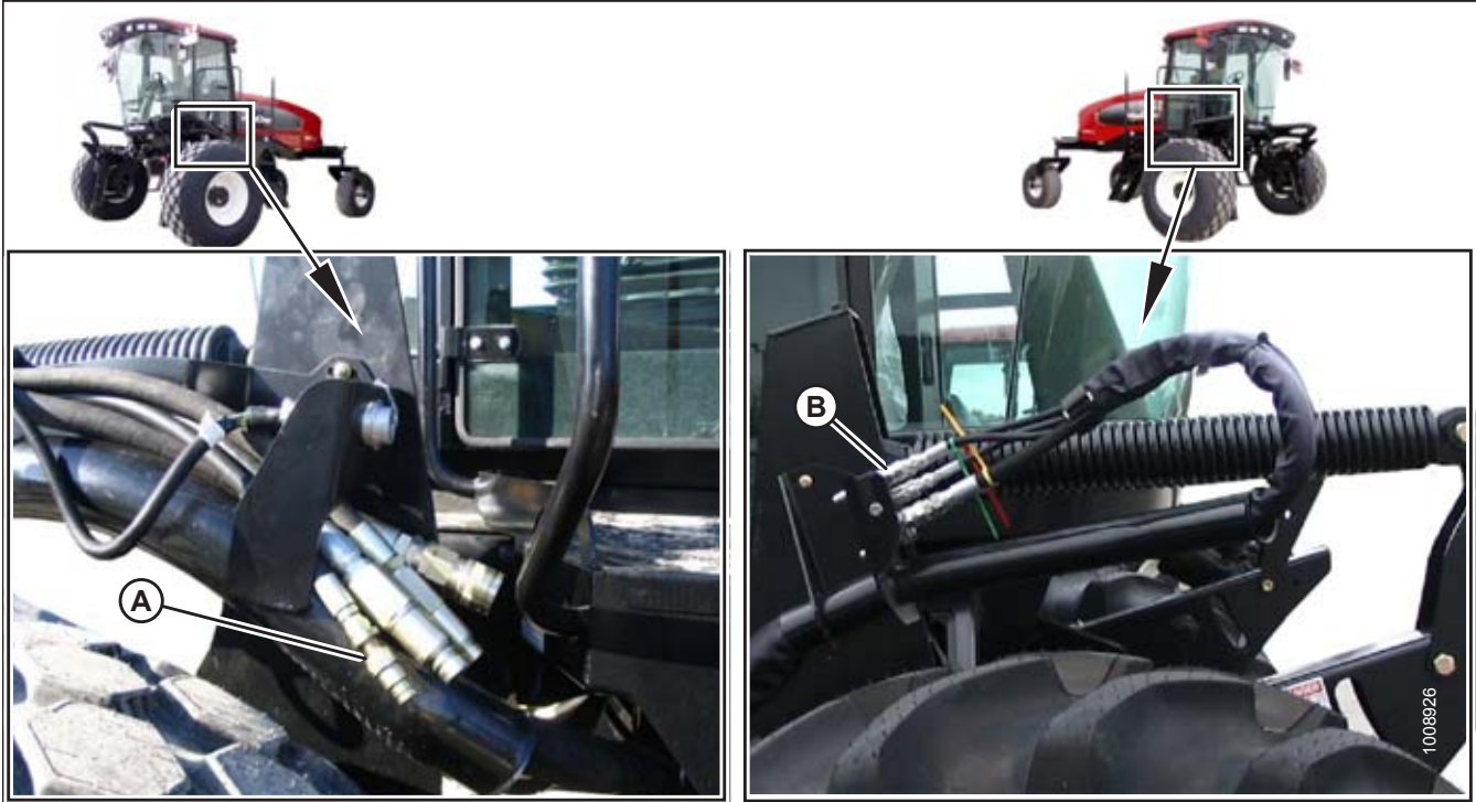
A - Header-Drive Hydraulics
