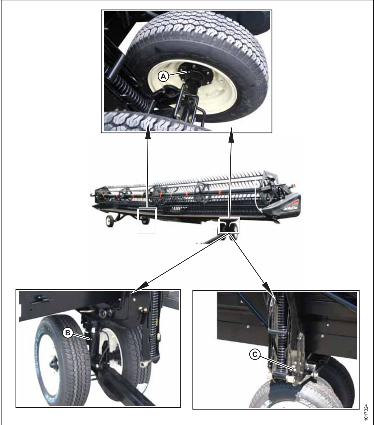
Figure 5.66: Rear Wheel Axle, Wheel Bearings, Frame/Wheel Pivot, and Front Wheel Pivot
