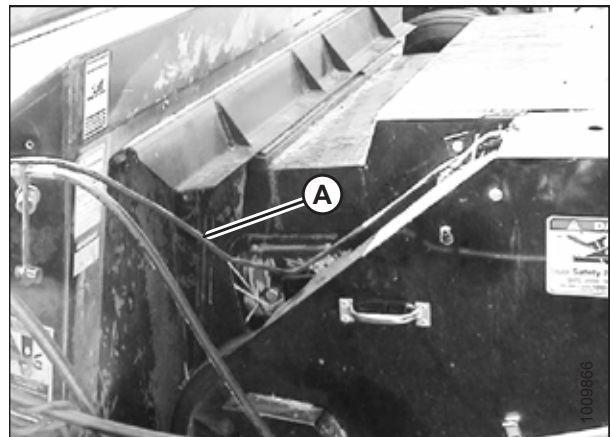
Figure 4.13: Switch Harness Routing
