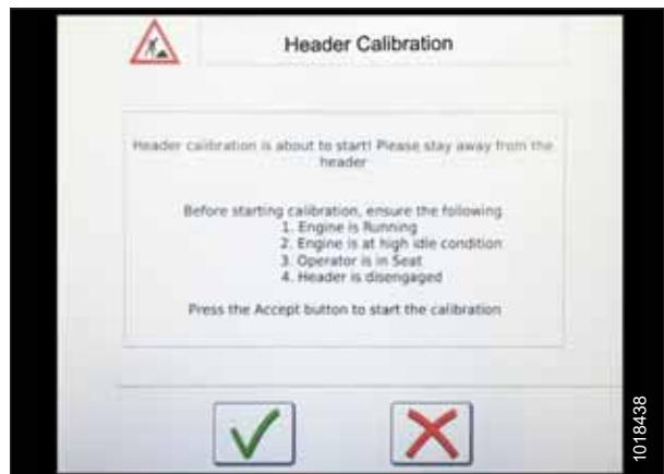
Figure 6.41: Header Calibration Warning
