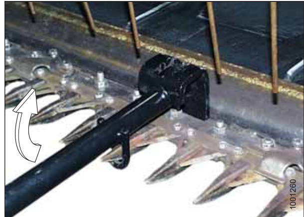
Figure 8.7: Straightening Tool – Upward Adjustment
