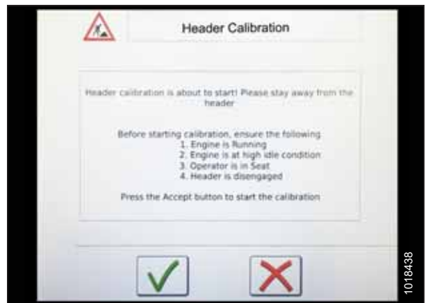
Figure 6.241: Header Calibration Warning
