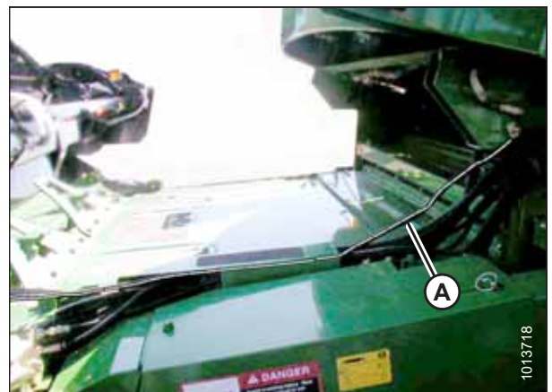
Figure 4.77: 60/70 Series Harness Routing
