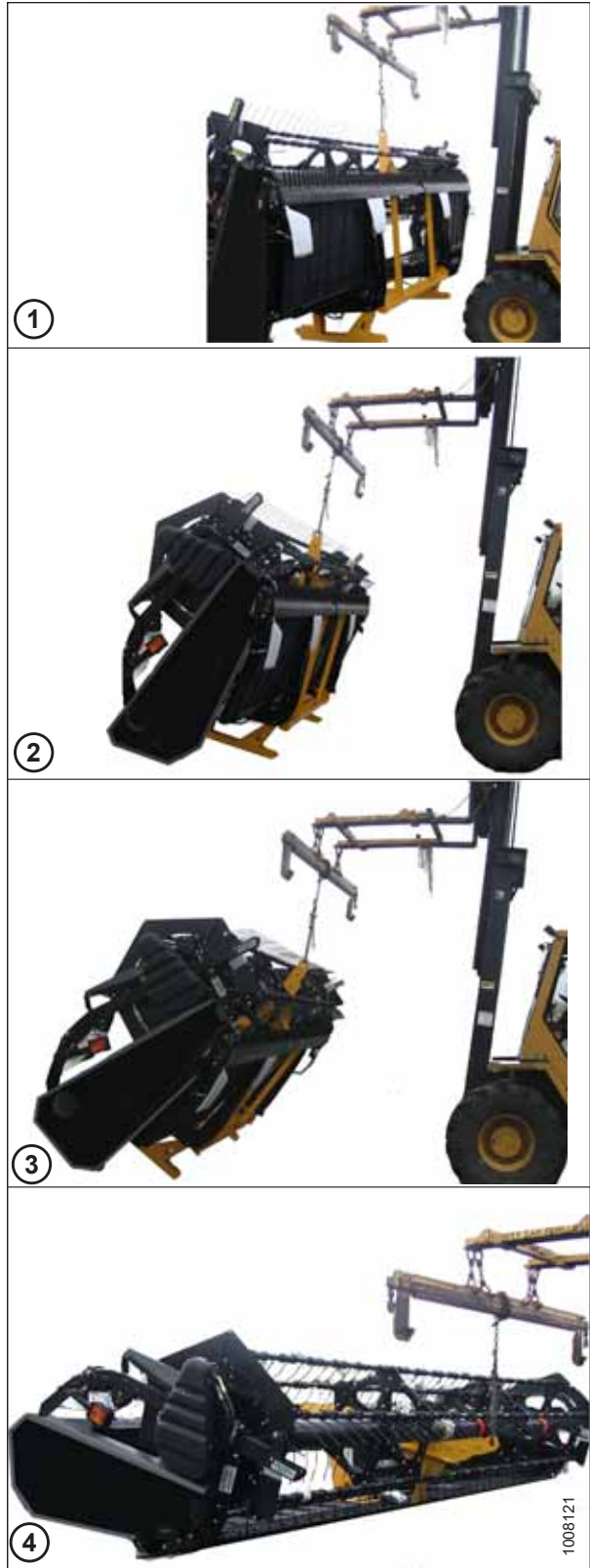
Figure 2.6: Header Lowered onto Ground
