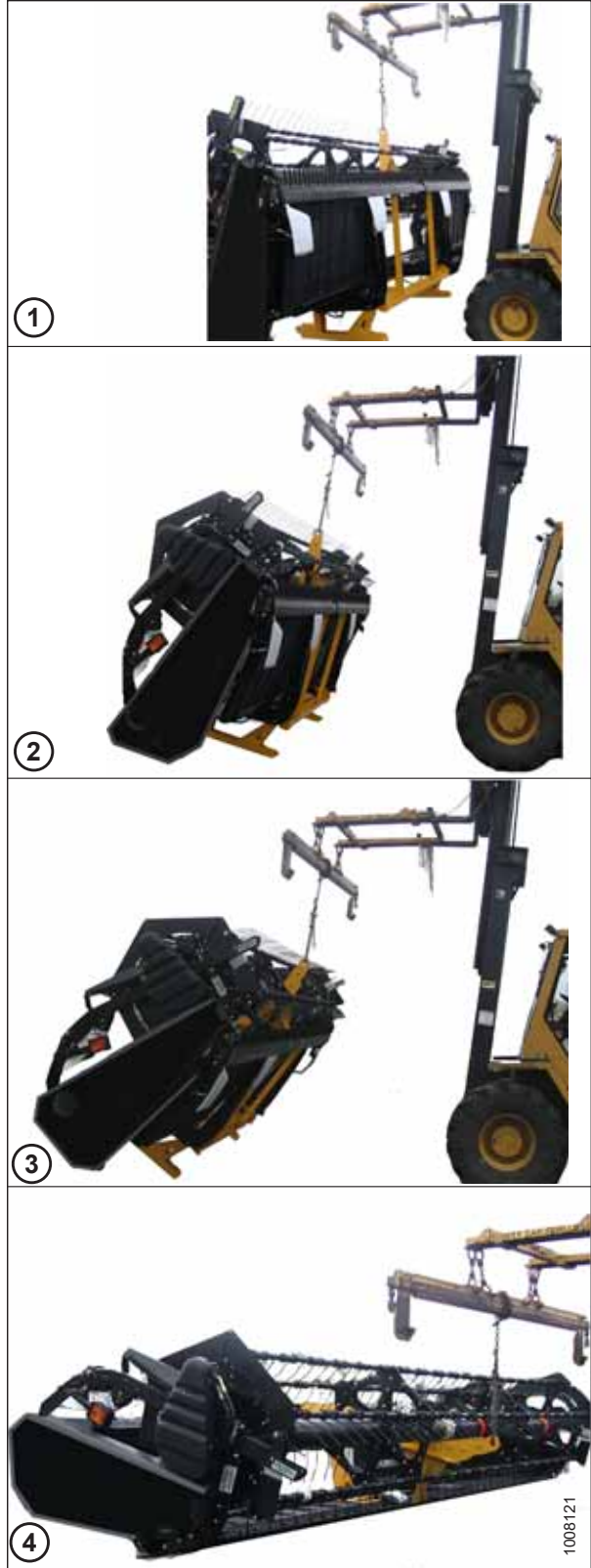
Figure 2.6: Header Lowered onto Ground
