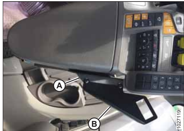
Figure 4.66: Top View of Armrest Showing Supports Installed in Preferred Location
