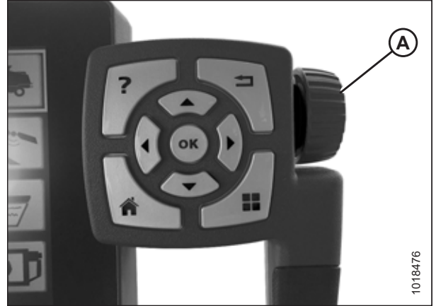
Figure 6.246: Adjustment Wheel on Right Side of Tyton Terminal
