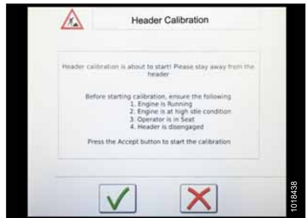
Figure 6.42: Header Calibration Warning
