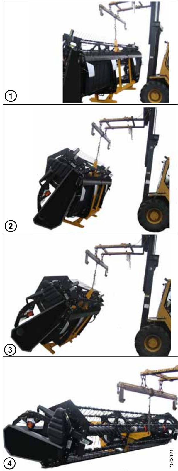
Figure 2.5: Header Lowered onto Ground
