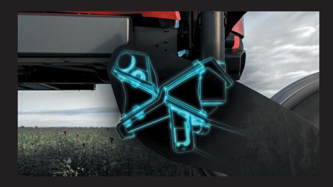
MacDon's patented CrossFlex™ Suspension makes in-field speeds up to 29 km/h (18 mph) possible, as this innovative design absorbs impact from rough terrain, allowing smooth harvesting no matter the field condition.
