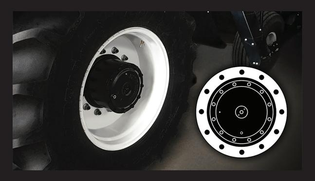
Order an M2 with the HT (High Torque) spec for those working in extremely hilly fields. These High Torque wheel drive units have a higher final drive ratio for increased drive wheel torque, allowing harvesting performance on slopes greater than 18 degrees (32% grade).\*
