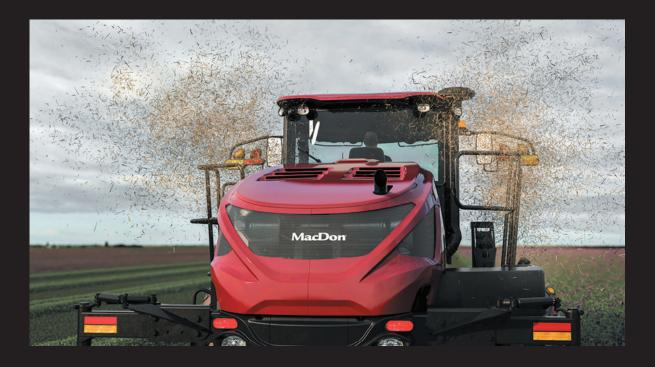
M2 Series Windrowers feature a dual radiator design. The cooling fan behind the cab pulls in clean air and kicks in to reverse independently to blow out debris from the radiator. This constant, fresh airflow keeps the engine and hydraulics running cool all day.
