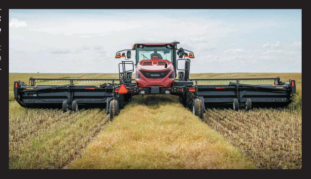
Featuring the Industry's best crop clearance with 115 cm (45") of height and 341 cm (134") of width, big bushy swaths flow effortlessly under M2 Series Windrowers.\* Ample header lift height lets you get up and over the tallest bushiest windrows with ease.
