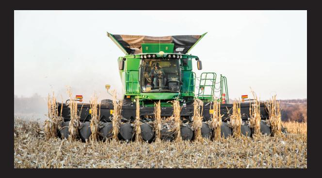
Seedbed preparation starts at harvest time. With a strong focus on agronomy, MacDon C and FC Series headers provide industry-leading residue management. MacDon's OctiRoll™ system creates well-conditioned, evenly chopped, and evenly distributed residue in a single pass - even in the toughest corn varieties. MacDon's thorough and consistent processing results in faster decomposition to maximize the potential for next year's crop.
