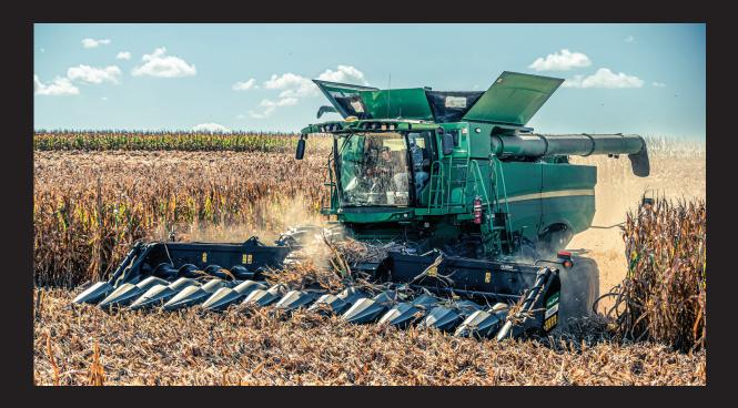
The two pivoting wings on MacDon's FlexCorn Header independently track steep terraces and uneven ground conditions for a more thorough and even cut of the trickiest patches of your field. Adjustable wing kick raises wings at the end of the pass to maximize turning maneuverability.
