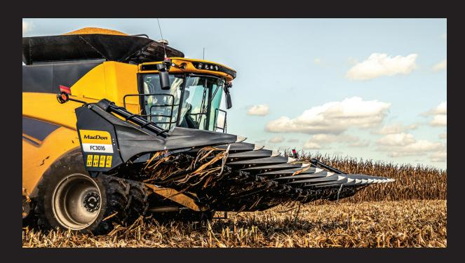
The FlexCorn wings have over 15 degrees of range, so a 16-row header with 30-inch (76.2 cm) spacing provides 61 inches (155 cm) of total flex range on each end.
