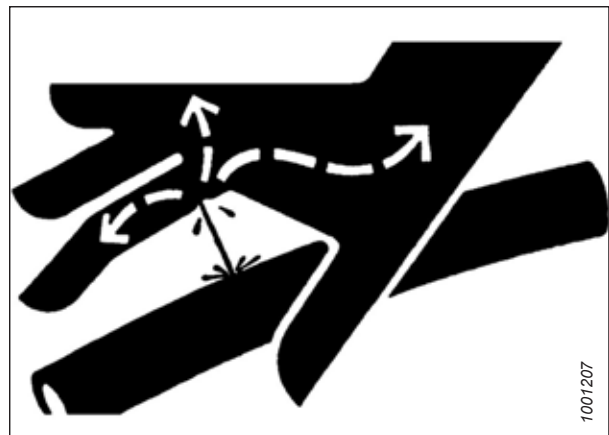
Figure 1.9: Hydraulic Pressure Hazard
