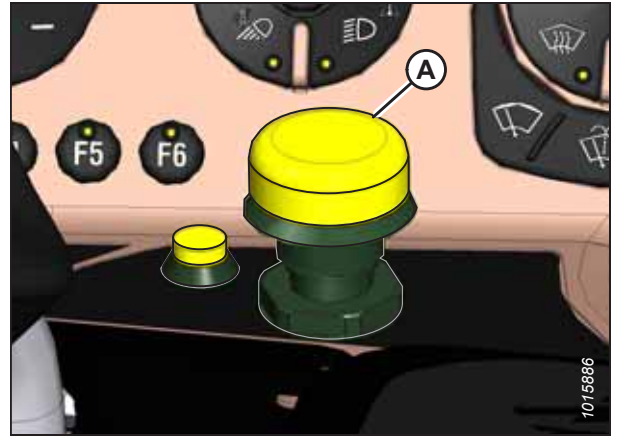
Figure 5.24: Header Engage Switch
