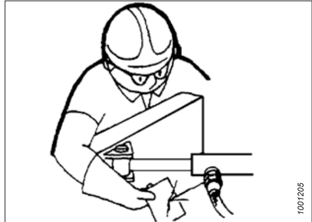
Figure 1.8: Testing for Hydraulic Leaks
