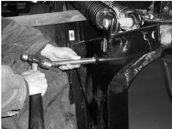
REMOVING RETAINING PIN
