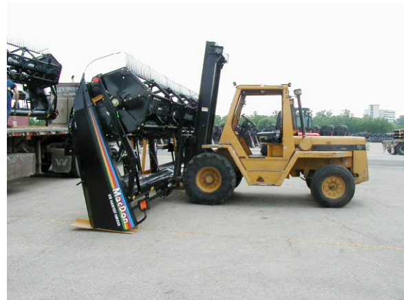
UNLOADING WINDROWER FROM TOPSIDE
