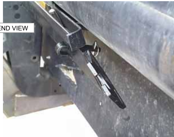
STEP 15: DIAGONAL BRACE & J-BAR STORAGE - 972
