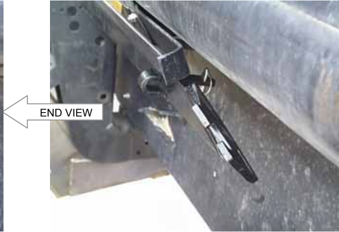
STEP 14: DIAGONAL BRACE & J-BAR STORAGE - 972
