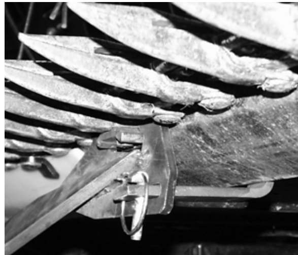
STEP 16: INSTALL J-BAR – 972 & 973 HEADERS
