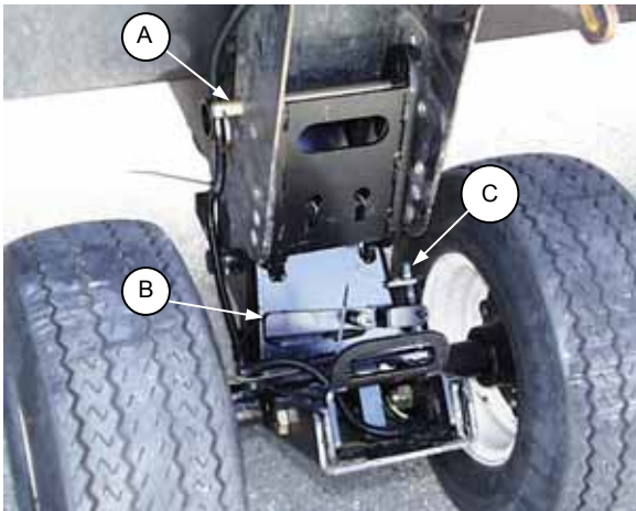
L/H WHEEL SUPPORT: FIELD POSITION
