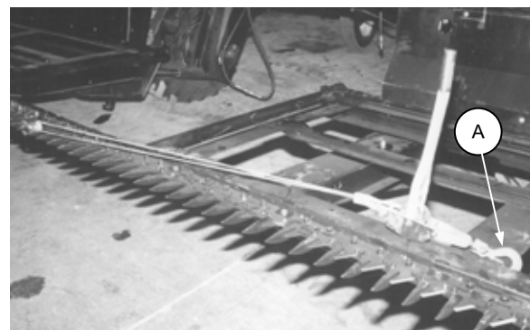
USE "COME-ALONG" TO MOVE DECK
