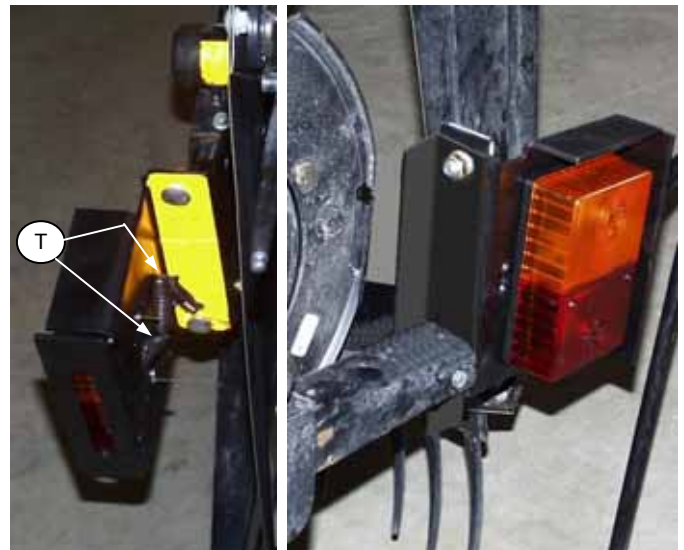
INSTALL LIGHTS AT R/H REEL SUPPORT ARM
