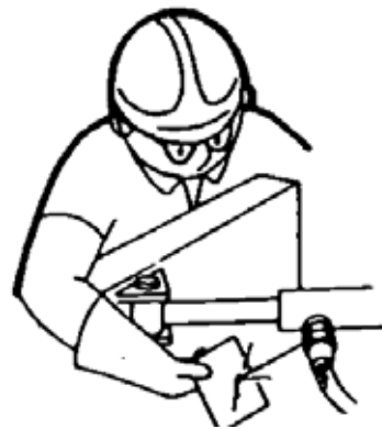
CHECK PROPERLY FOR LEAKS
