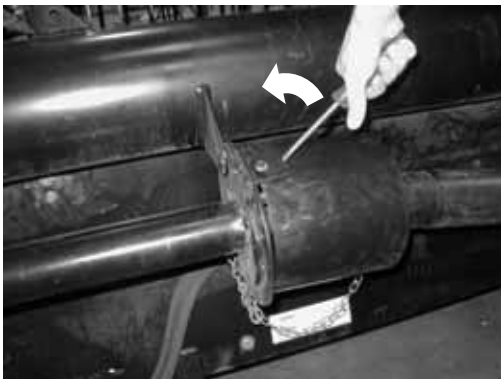
REMOVING DRIVELINE SHIELD
