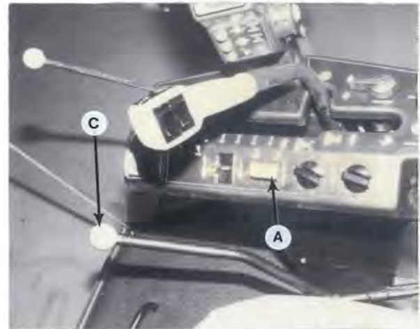
HEADER DRIVE SWITCH OFF & SPEED-RANGE CONTROL TO "ROAD"
