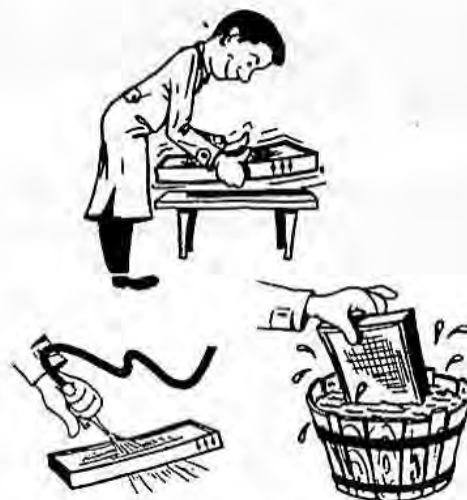
CLEANING AIR FILTER
