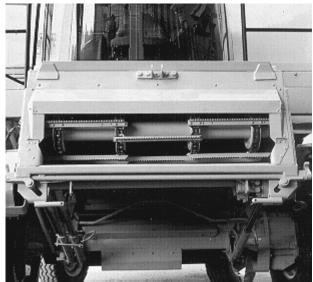
1.) Remove feeder house top, L/H and R/H dust shields.
