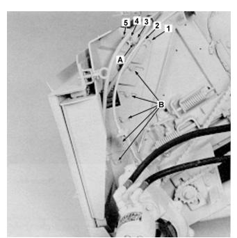
5.) Adjust Feeder House faceplate back.-Tilt face plate rearward to mid-position.
