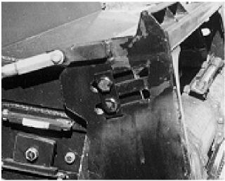
4.) Tilt feeder house face plate back at least ¾ of the way.
