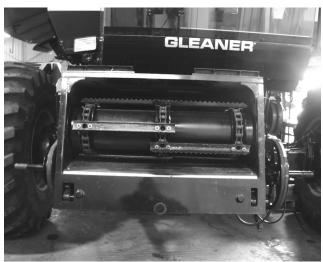
1.) Remove feeder house top, L/H and R/H dust shields.
