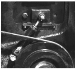
3.) Set feed conveyor drum height to small grains position as per combine operators manual.
