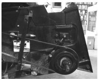
5.) Set feeder house drive output speed to 625 rpm.
