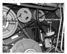
Combine must be equipped with reel drive pump located on the L/H combine side panel.
