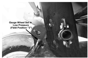
For crop stubble 8" (210mm) or less, set gauge wheels/transport to low pressure (field position "2").
