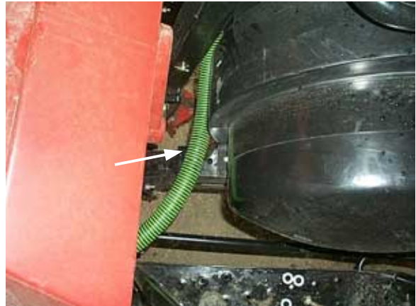
VENT LINE ATTACHED TO REAR TANK
