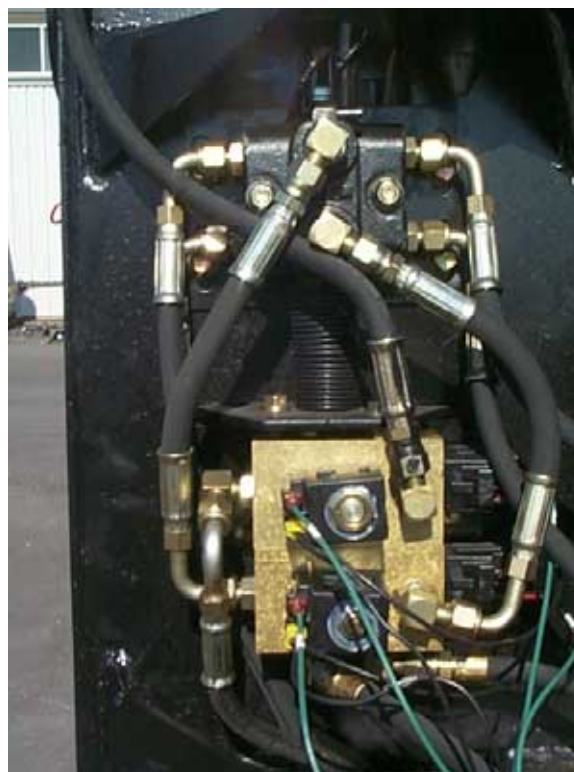
MAST SOLENOIDS & SELECTOR VALVE
