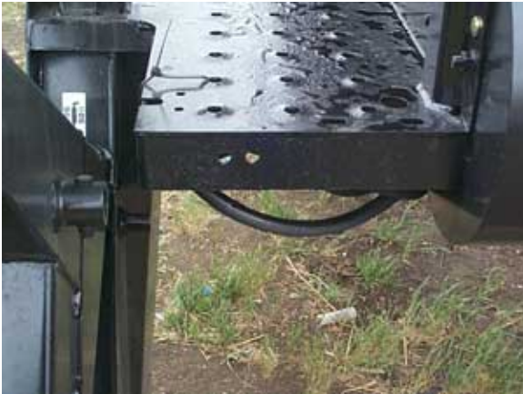
L/H HOLES FOR DECK SUPPORT
